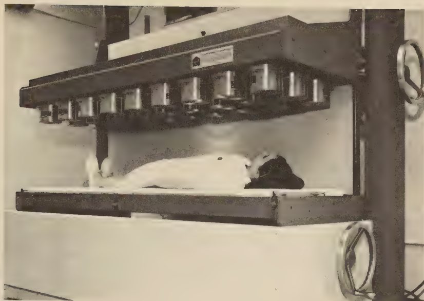
A nurse simulates a patient being scanned by a whole-body counter consisting of 54 sodium-iodide crystal detectors. (27 above, 27 hidden below the patient.) Rather than scanning the patient with a single moving detector, this whole-body scanner creates two 27-element pictures simultaneously. ( Brookhaven National Laboratory )
