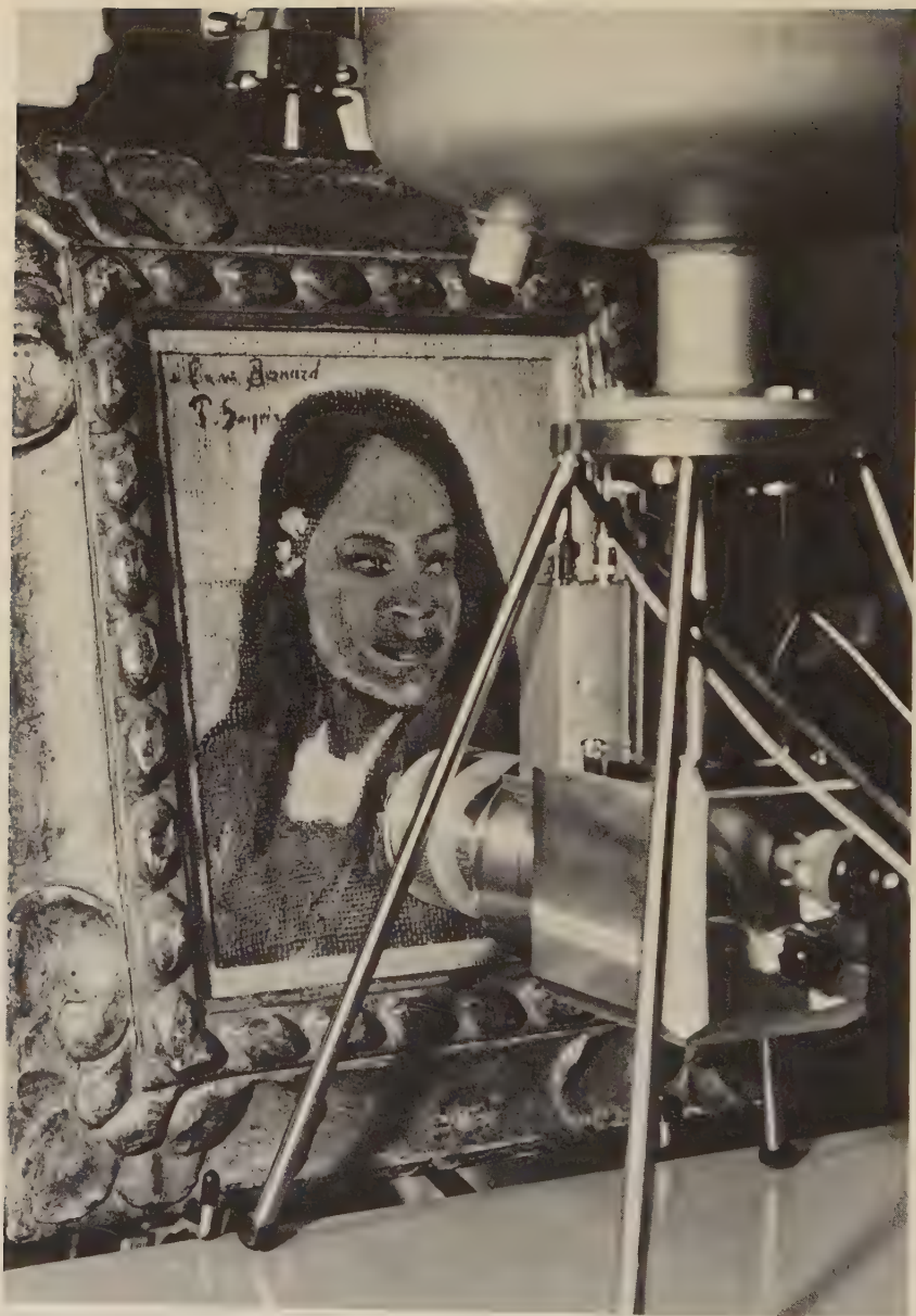
X-ray fluorescence equipment being used to study a Gauguin painting. X-ray fluorescence is nondestructive and very helpful in checking the authenticity of valuable paintings and archeological finds. (Kevex Corporation)
