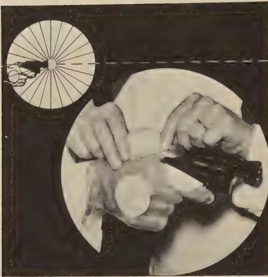
Minute quantities of gunpowder residue from muzzle flashback can often be detected on a suspect's hand by activation analysis. Frequently, the powder manufacturer can be pinpointed. ( U.S. Atomic Energy Commission. )
