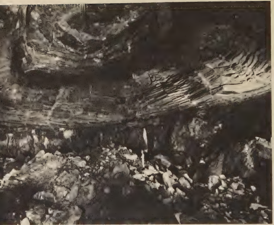
The hemispherical cavity created by the Gnome explosion was about 75 feet high and 134 to 196 feet across. Note the man standing on the rubble at right center. ( U.S. Atomic Energy Commission )
