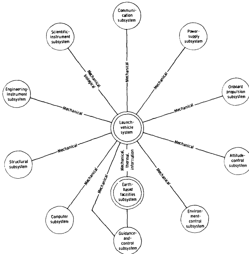
FIGURE 8-2.—Interface diagram showing the more important relationships between the launch vehicle and the rest of the satellite system.
