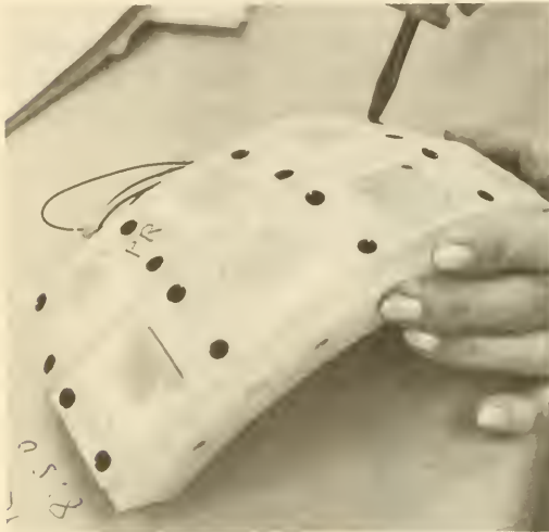
FIGURE 14-8.—Assembling one of the two Drosophila packages to be flown on Biosatellite A/B. Each package has eight cubical modules holding flies and agar nutrient.
