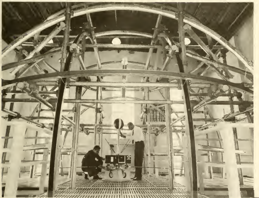
FIGURE 7-13.—The Magnetic Field Component Test Facility at Goddard Space Flight Center. The large external coils can null out the Earth's field, which, at sea level, is many times larger than the fields to be measured in space. Residual spacecraft fields can be mapped and instruments calibrated.
