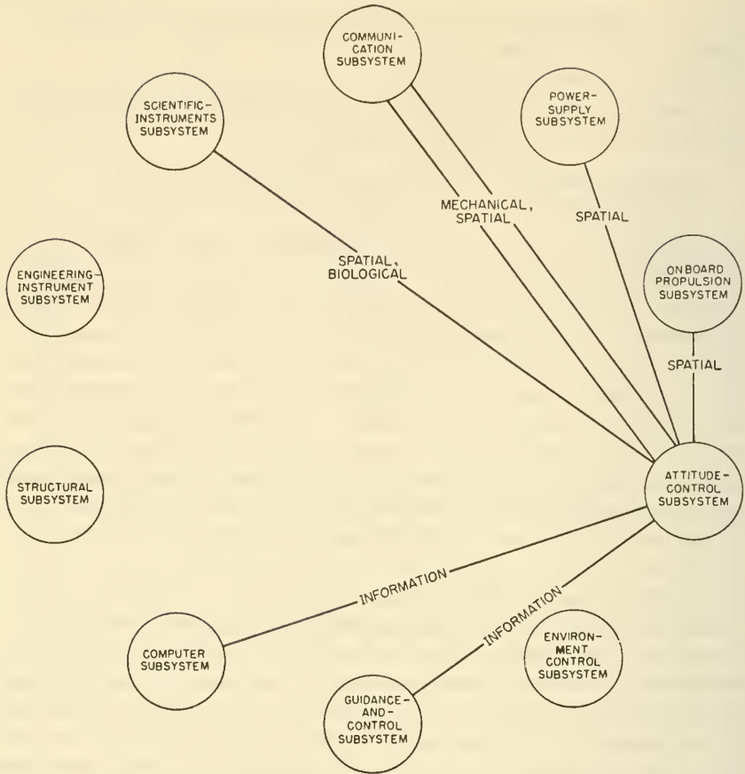
FIGURE 9-45.—Portion of the satellite-interface diagram showing the relationship of the attitude-control subsystem to the rest of the satellite.
