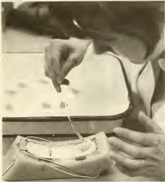
FIGURE 14-7.—Loading flour-beetle larvae ( Tribolium ) into Biosatellite-A/B experiment package. Wires are for strip heaters.
