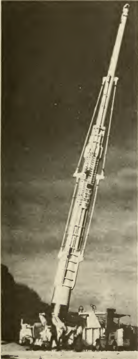
FIGURE 8-11.—A reborescoped, 16-inch Navy cannon used for firing high-altitude research probes from Barbados Island, B.W.I. Small satellites could also be launched with such a gun.
