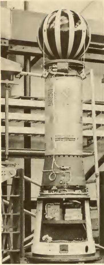
FIGURE 7-17.—San Marco 1 and the Scout fourth stage undergoing a spin test at Wallops Island.
