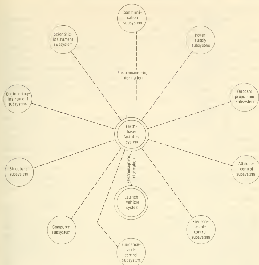
FIGURE 7-1.—Interface diagram showing the more important relationships between the Earth-based facilities and the rest of the satellite system. The dotted lines represent prelaunch testing and checkout relationships; the solid lines show postlaunch interfaces.
