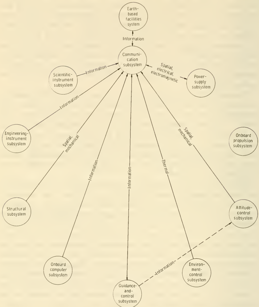
FIGURE 5-2.—Interface diagram showing the more important relationships between the communication subsystem and the rest of the spacecraft. The dotted line shows one of the many other information links that bypass the communication subsystem.
