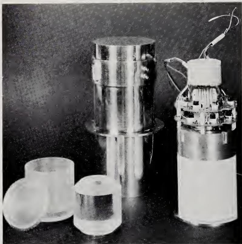
Fig. 15-18. The Ranger-3 gamma-ray spectrometer disassembled. (Courtesy of the Los Alamos Scientific Laboratory)
