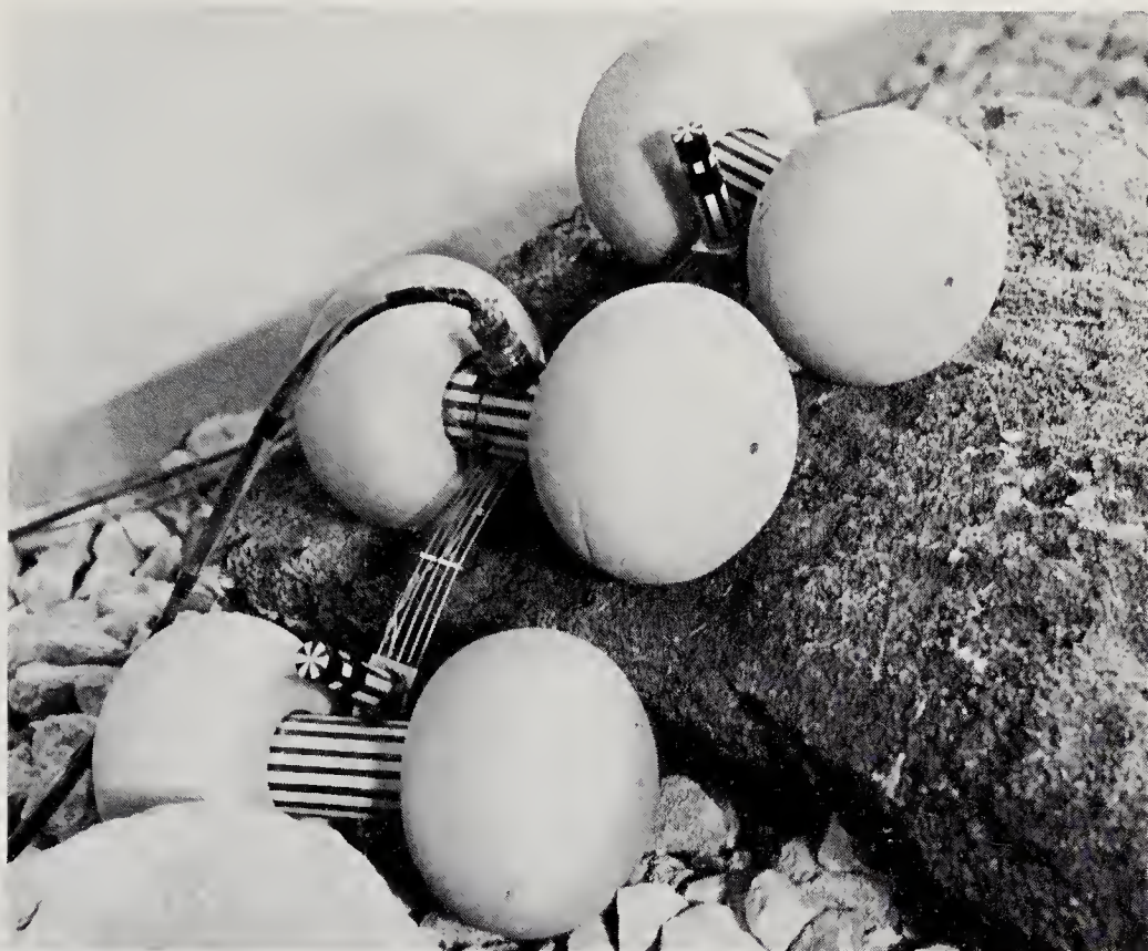
Fig. 10-17. Flexibly connected, doughnut-wheeled vehicle for locomotion on planetary and lunar surfaces. (Courtesy of General Motors Corp.)
