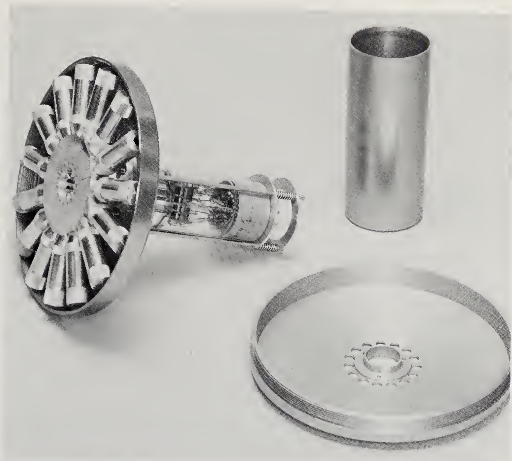
Fig. 16-13. One of the Multivator prototypes. This model shows fifteen reaction chambers and a photomultiplier tube, which is used with those chambers employing light signals. Dust and aerosol samples are blown into the radial chambers. (Courtesy of Stanford University)
