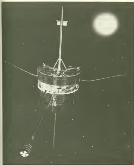
FIGURE 2-3.—View of the Pioneer spacecraft showing the three radial booms deployed, the telemetry antenna mast (top), and the Stanford radio propagation experiment antenna (bottom).
