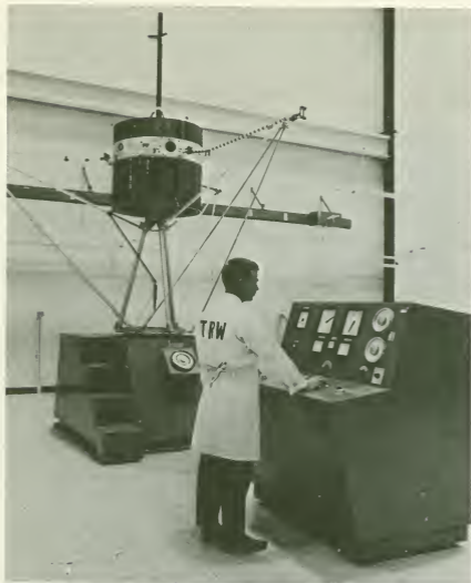
FIGURE 3-5.—The Pioneer-6 spacecraft, showing final boom arrangement and the viewing band void of solar cells. Spacecraft is undergoing a spin test.
