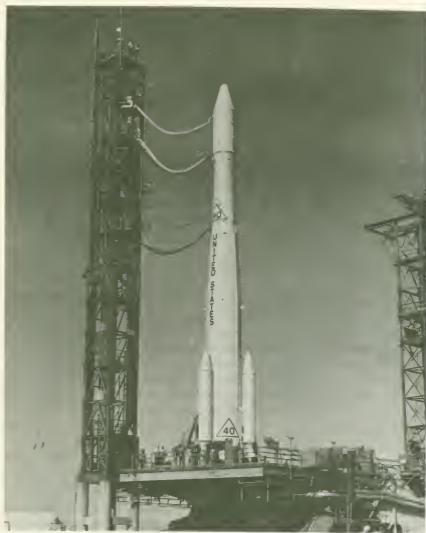
FIGURE 7-1.—The Pioneer-7 launch from Complex 17A at Cape Kennedy. Delta 40 was a thrust-augmented improved Model E launch vehicle.
