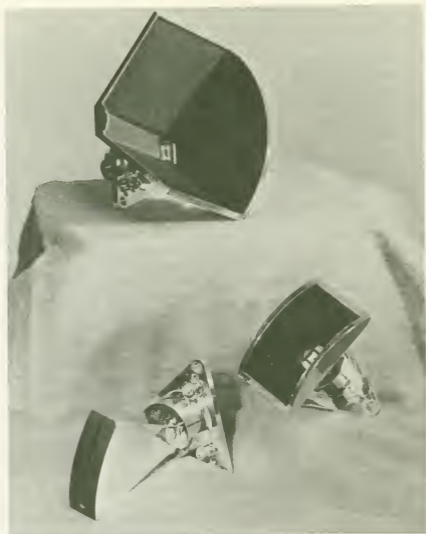
FIGURE 4-21.—The Pioneer Sun sensors: A or C (top); B or D (middle); and E (bottom).
