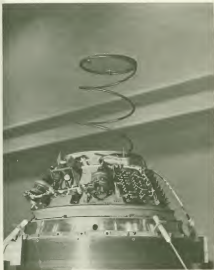
FIGURE 7-4.—The 9 × 8-in. conical attach fitting used on Delta Pioneer launches.
