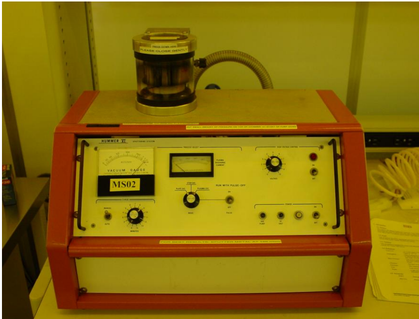
Figure 6. Hummer VI sputter deposition system for coating insulating SEM samples.
