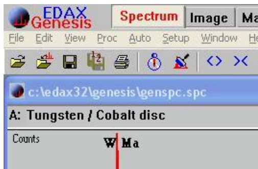
Figure 33. Spectra Title entry after the “A:” character at the upper left corner of the spectra window.
