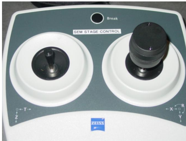
Figure 11. Joystick Stage control. LEFT stick performs stage Z-travel and Tilt: Z-travel – push lever up or down; Tilt – push the lever right or left. RIGHT joystick moves stage in x and y and twisting the right stick causes the stage to rotate.
