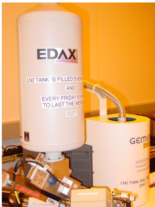
Figure 24. EDAX LN 2 Dewar and pre-amplifier mounted on the Gemini electron microscope column.
