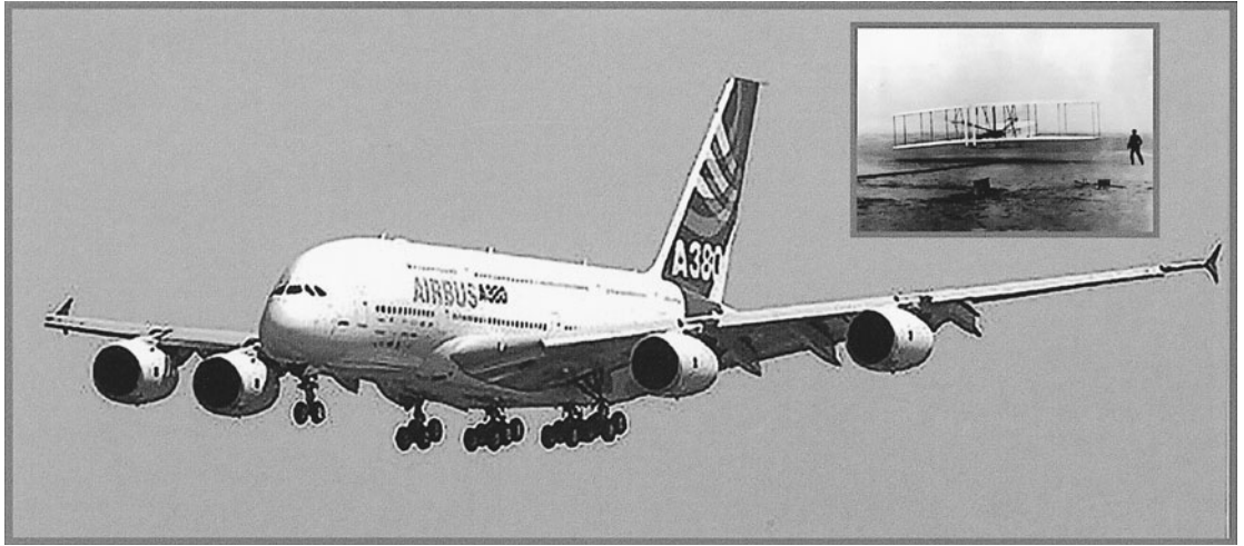
Fig. 17.2. A century of flight. The world's largest passenger plane, the Airbus A380, on its maiden flight, April 27, 2005. Inset (to scale): The Wright brothers' first flight at Kitty Hawk, North Carolina, on December 17, 1903. The A380 has a wingspan six times that of the Wright brothers' flyer and, fully loaded, weighs over two thousand times more.
