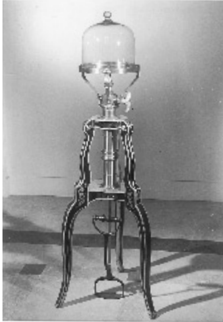
Figure 22.1. An air pump made for Jean-Antoine Nollet (1700–1770), the successful French scientific lecturer and deviser of demonstration apparatus. The instrument is decorated in the ornate, black-and-gold style that is typical of Nollet.
