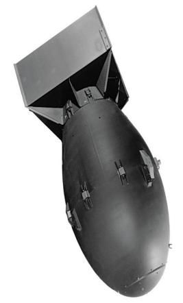
"Fat Man," the atomic fission bomb dropped over Nagasaki, Japan, on August 9, 1945. The bomb consisted of a slightly sub-critical mass of plutonium encased by chemical high explosives. It was 3.3 meters (10.8 feet) long and had a yield of 21 kilotons—equivalent to 21,000 tons (23,000 tons) of TNT.
