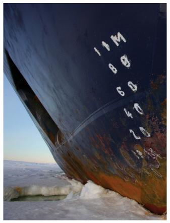
Iron, and steel (which is an alloy of iron and carbon), are both susceptible to corrosion—an "oxidation" reaction, where iron reacts with oxygen to formiron oxide, also known as rust. The steel hulls of ships can be protected from corrosion by being "galvanized" with a zinc coating.
