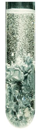
This reaction between pieces of zinc metal and hydrochloric acid produces bubbles of hydrogen. Hydrochloric acid molecules are made of hydrogen and chlorine atoms.
