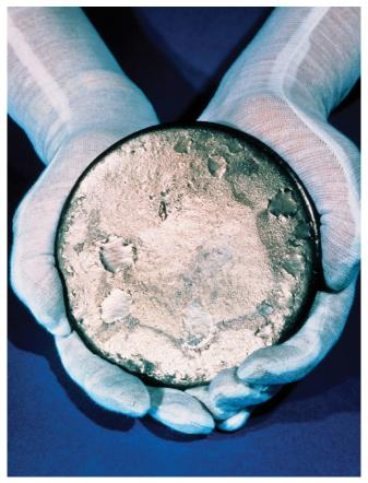
A "button" of uranium-235, the radioactive isotope that is used as a fuel for nuclear reactors and as an explosive in nuclear weapons, such as the Hiroshima bomb. It weighs about 4.5 kg (almost 10 lb) and is worth approximately US\$200,000.
