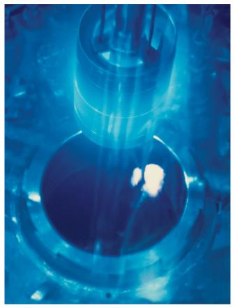
A nuclear fuel rod is removed from the High Flux Isotope Reactor (HFIR) at Oak Ridge National Laboratory, USA. The 100-megawatt reactor produces a very high neutron flux and is used to conduct research on man-made elements heavier than plutonium. Its principal product is the synthetic isotope californium-252.
