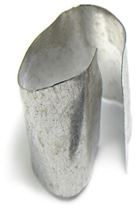
A strip of indium foil. The rare, soft malleable metal is used inside computers as an interface material between microchips and their heat sinks to dissipate thermal energy and prevent the chips from overheating.
