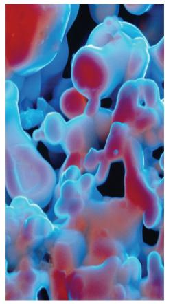
superconductor. This superconducting metal material is made up of lanthanum, barium and copper oxide. Superconductors carry electrical current with little or no resistance. The phenomenon occurs in certain materials at very low temperatures (just a few degrees above absolute zero), where the atoms in the material undergo a change allowing the electrons that carry electric current to slip past unimpeded.
