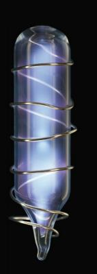
Argon gas in a borosilicate vial. Like the other noble gases, argon is used in discharge lamps, where it is made to glow by passing an electric current through it.
