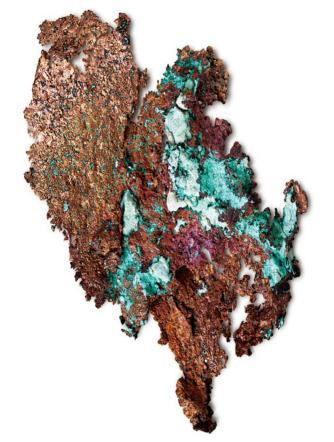
Unmixed native copper in its oxidized state. The corroded parts have a green hue.
