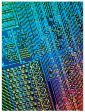
Pictured is a light micrograph of a silicon microchip. Microchips are made from wafers of silicon, "etched" with conducting channels and regions of enhanced positive and negative charge to give them the required electrical properties.
