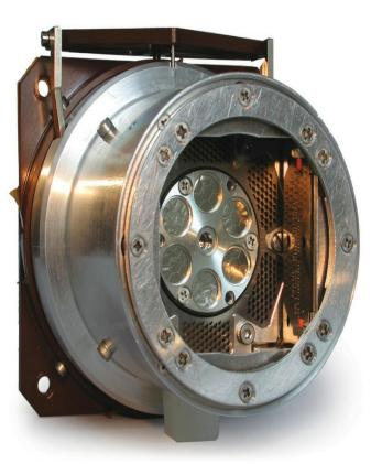
The Alpha Particle X-Ray Spectrometer (APXS) used on NASA's Mars Exploration Rover mission. This device uses small amounts of curium-244 to determine the concentrations of major elements in rocks and soil. It does so by bombarding samples with alpha particles given offby the curium. The paths of the alpha particles as they bounce back, and the energy of X-rays produced as the particles collide with electrons, tell scientists what the sample is made from
