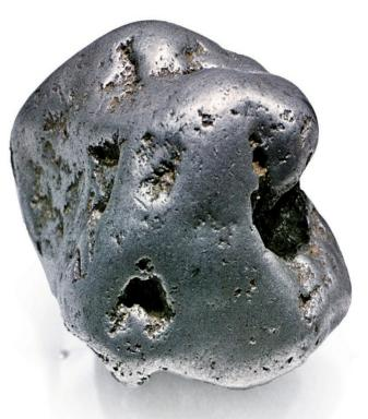
Pictured is a platinumnugget weighing 5.918 kg (13 lb)—worth, to its lucky owner, more than US\$300,000 (at 2013 prices). Platinum is not only a precious metal, but it is also an essential component of automotive catalytic converters.
