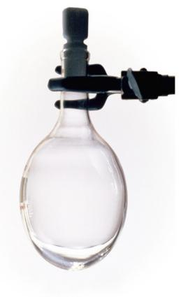
Xenon is a colorless, odorless, inert, noble gas. Hard to believe, then, that it's used as rocket fuel. A relatively new formofrocket called an "ion engine" uses an electric field to accelerate charged xenon atoms to forma high-speed exhaust jet that can propel a vehicle through space.
