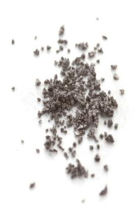
Having one of the highest melting points of all elements, rhenium is mostly combined with nickel and tungsten to form corrosion-resistant alloys that have excellent strength, even at very high temperatures.
