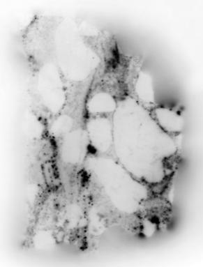
Traces of actinium can be isolated from pitch blende, a type of radioactive uranium ore. This image was produced by placing pitch blende on a sheet of sensitive X-ray film for four days. The darkest spots represent the highest sources of radiation.
