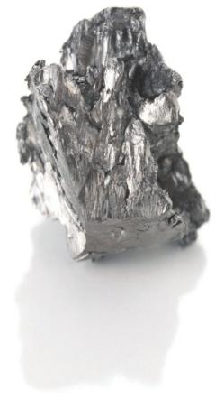
Dysprosium is a soft, silvery metal. Its applications include high-power magnets, neutron-absorbing control rods in nuclear power plants, radiation dose meters and high-intensity commercial lighting.
