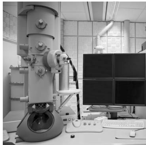
Electron microscopes utilize a beam of electrons emitted by a heated tungsten filament as the source of illumination.
