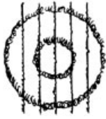
Figure 10.16: Diffraction pattern of two circular holes.
