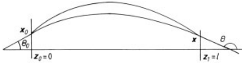
Figure 8.8: Imaging a small surface segment F_0 orthogonal to the optic axis at z_0 = 0 onto a surface segment F_1 at z_1 = l .
