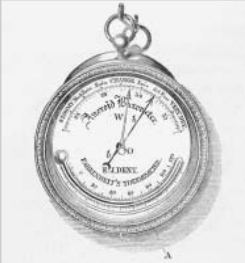
A drawing of an early aneroid barometer used to predict changes in the weather. National Oceanic and Atmospheric Administration. Reproduced by permission.
