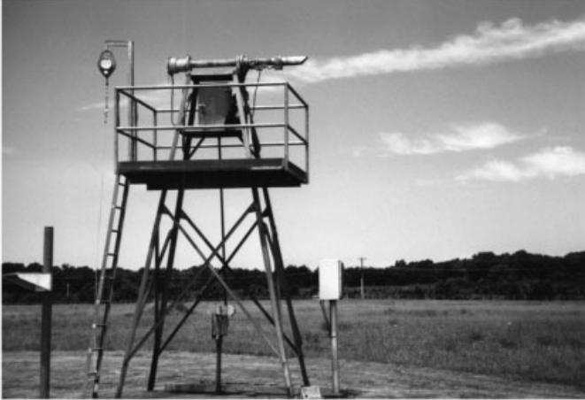
**Figure 19** Transmissometer. See ftp site for color image.
