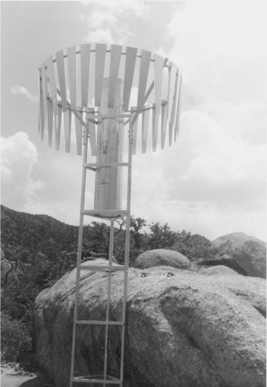
**Figure 4** Alter wind shield on a tower-mounted precipitation gage (from Doesken and Judson, 1997).
