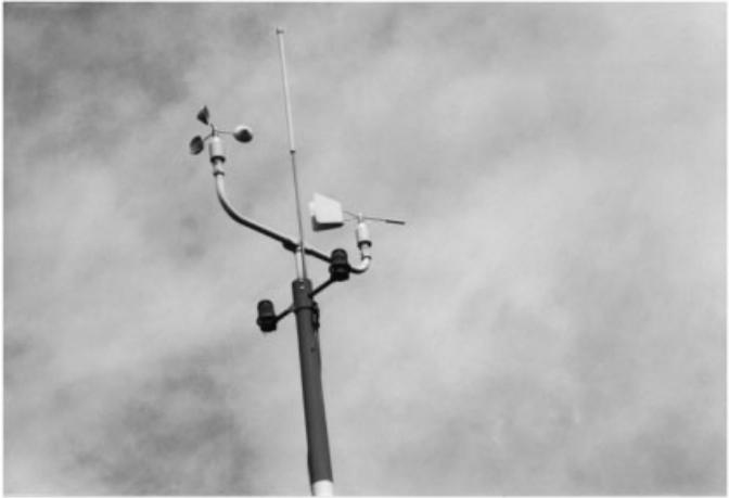
**Figure 11** Rotating cup anemometer and wind direction sensor atop 10-m tower. See ftp site for color image.
