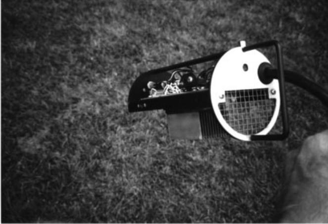
**Figure 5** Hygrothermometer interior showing intake air screen. Finned object on bottom is Peltier device. See ftp site for color image.
