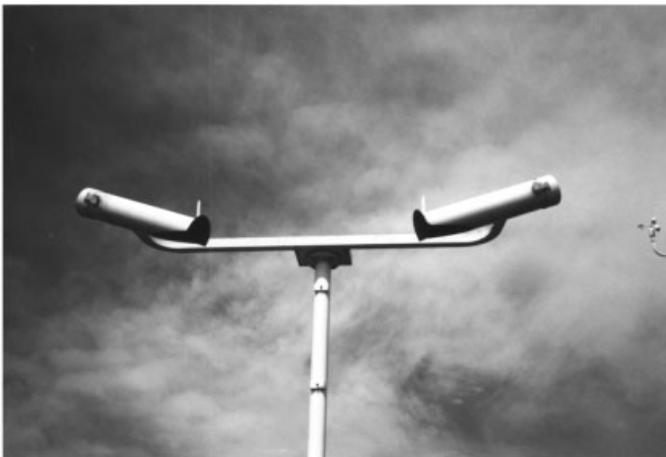
**Figure 20** Forward scatter visibility sensor showing projector and receiver. See ftp site for color image.
