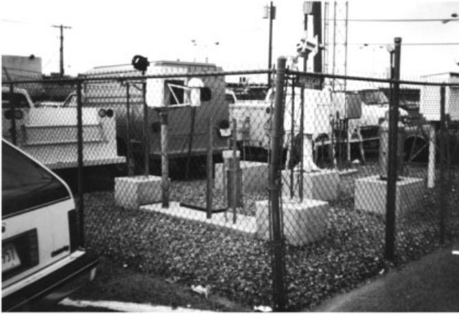
**Figure 25** Sensors poorly exposed in a parking lot. See ftp site for color image.
