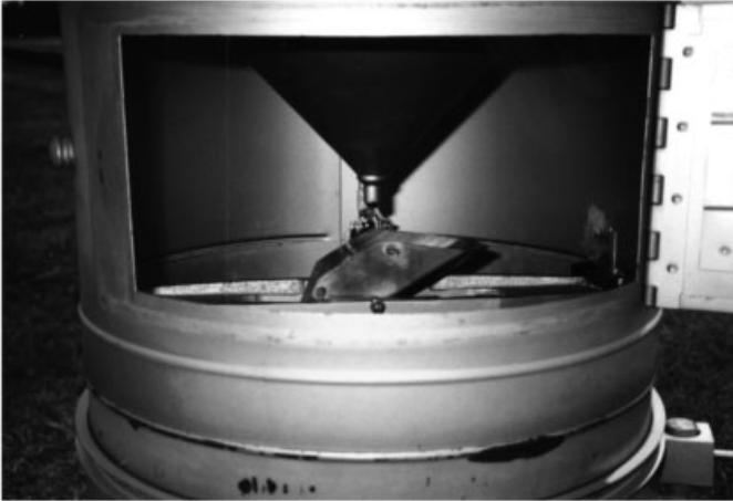
**Figure 8** Tipping bucket mechanism. See ftp site for color image.
