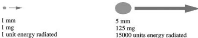
**Figure 5** Relative diameter, mass, and scattered energy from small and large drops. Large drops scatter much more energy than small drops. See ftp site for color image.
