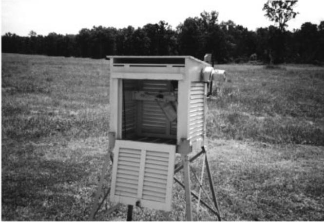
**Figure 2** Cotton Region temperature shelter with door open. See ftp site for color image.
