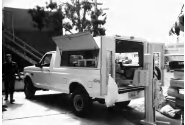
Figure 3. Direct push technology rig (Courtesy FAST-TEK).
