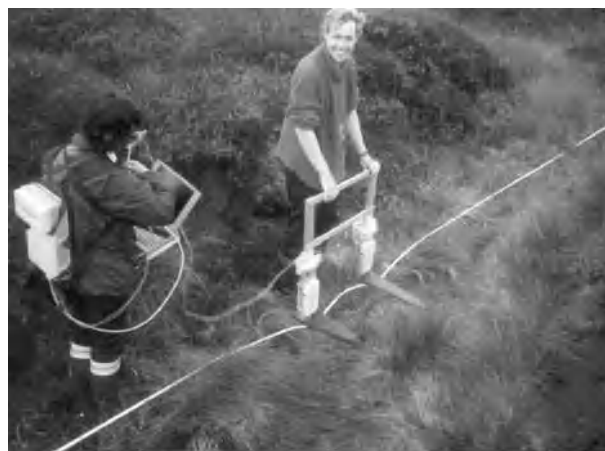
Figure 2. Ground penetrating radar being used in the field to detect soil pipes. Photo by Vincent Holden.
