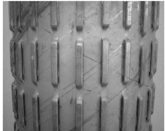
Figure 3. Bridge slot screen.
