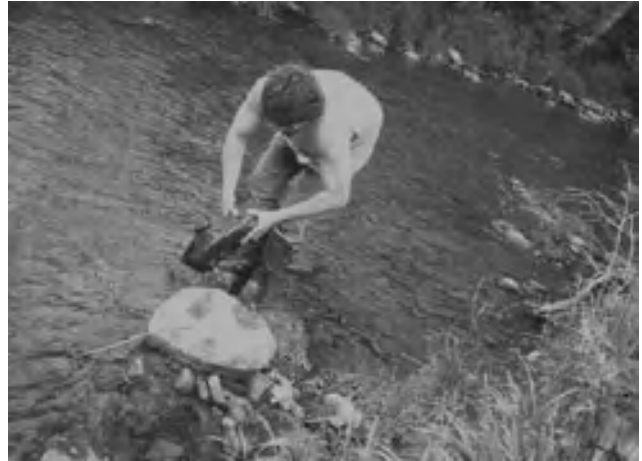
Figure 2. Activated charcoal packet attached to rock prior to placement in Waites Run, Hardy County, West Virginia.
