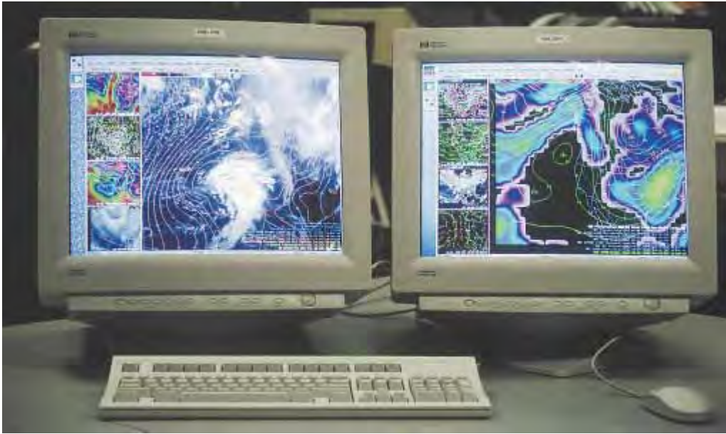
FIGURE 9.2 The AWIPS computer work station provides various weather maps and overlays on different screens.
