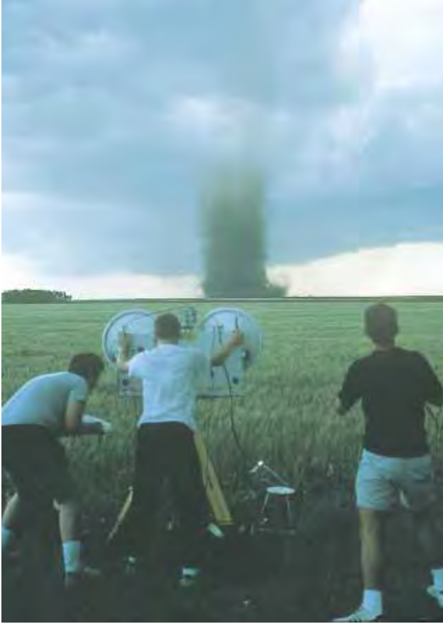
FIGURE 10.37 Graduate students from the University of Oklahoma use a portable Doppler radar to probe a tornado near Hodges, Oklahoma.
