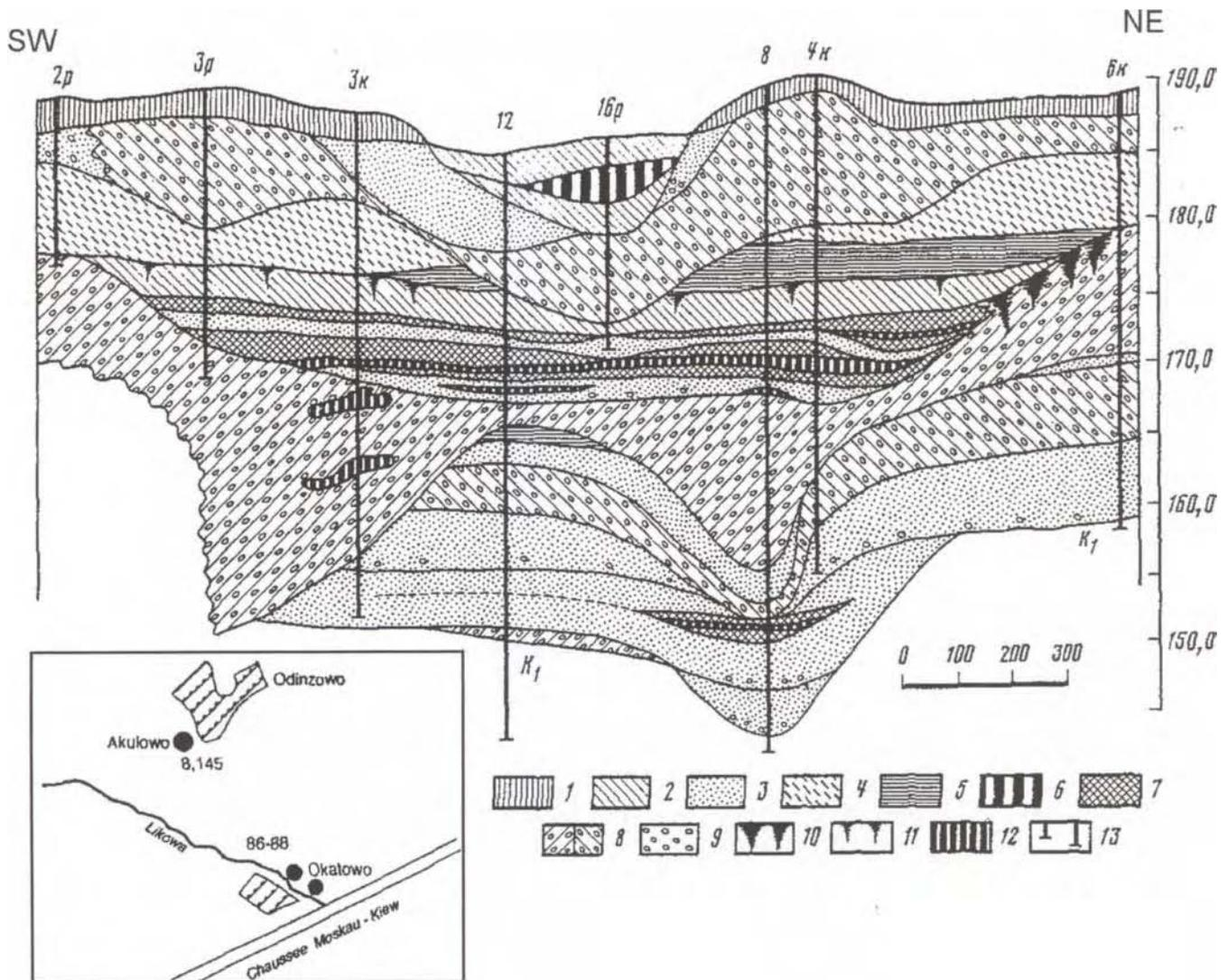
Fig. 2. Longitudinal section of the Akulovo site.
