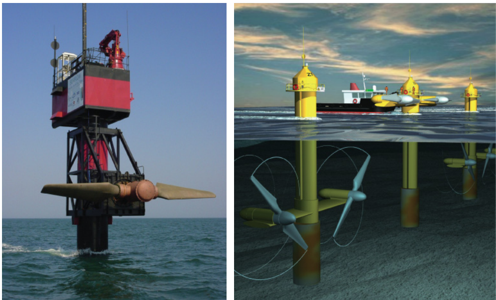
Figure 9.14 Left: Prototype system in Project Seaflow off the west coast of England. Photo: ISET. Right: Maintenance ship in a planned ocean current power plant park. Graphics: MCT.
