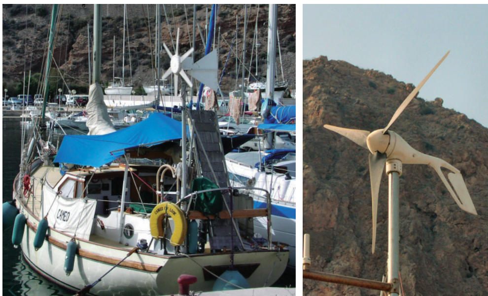
Figure 8.7 Small wind turbines used to charge battery systems.
