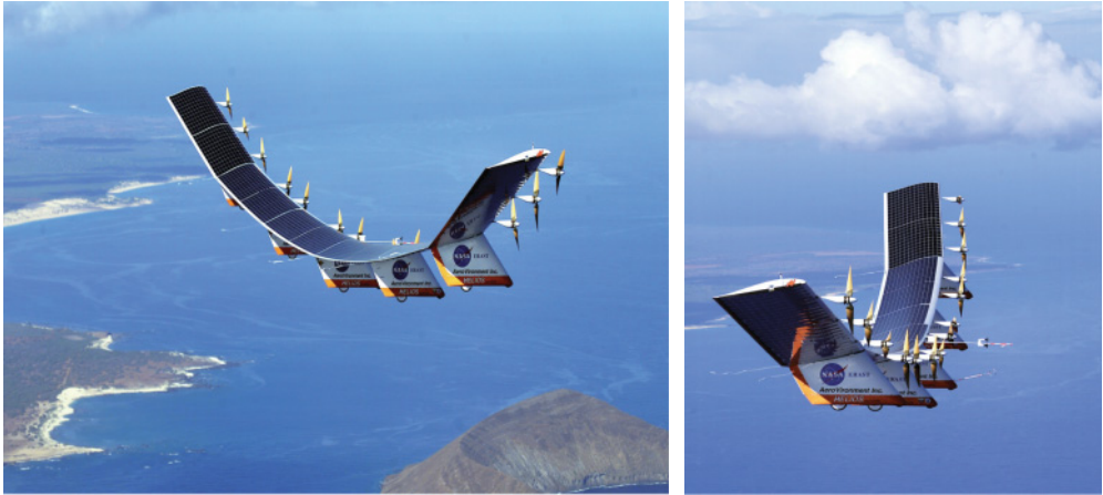
Figure 14.15 NASA's Helios aeroplane, powered only by solar cells, set a new world record for altitude in 2001. Photos: NASA, www.dfrc.nasa.gov .
