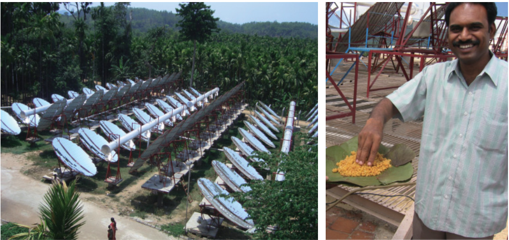
Figure 14.17 Solar-mirror systems financed through contributions from environmental protection funds replace conventional diesel burners in large kitchens in India. Source: atmosfair, www.atmosfair.com .
