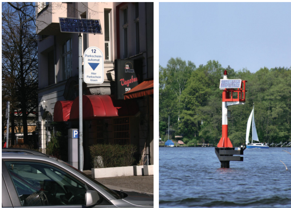
Figure 5.8 Photovoltaic island systems offer advantages for many applications compared to grid connections.
