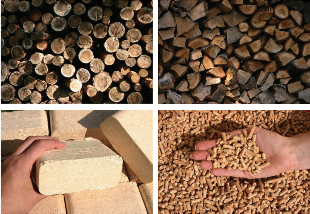
Figure 12.5 Different processed forms of wood. From top left to bottom right: round wood, firewood, wood briquettes, wood pellets.
