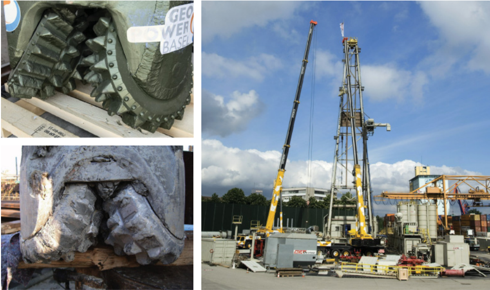
Figure 10.5 Left: New and used drill bits. Right: Structure of a derrick. Photos: Geopower Basel AG.
