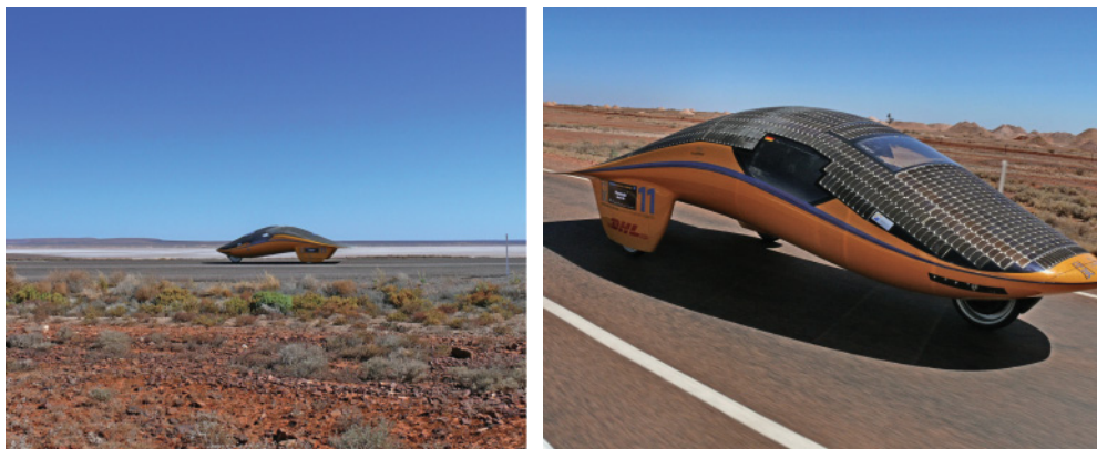
Figure 14.11 In 2007 the solar car from Bochum University reached average speeds of 73 km/h during the 3000 km race. Photos: Bochum University of Applied Sciences, http://www.hs-bochum.de/solarcar.html .
