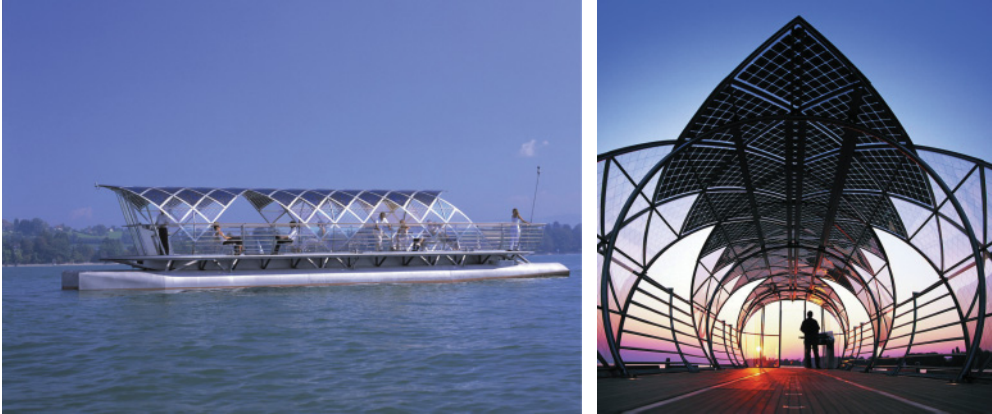
Figure 14.14 The Helio solar ferry has been crossing Lake Constance since 2000. Photos: Bodensee-Solarschiffahrt, www.solarfaehre.de .
