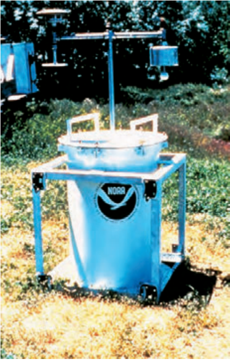
ATOTable Tornado Observatory (or TOTO) is placed in the path of oncoming tornadoes to measure air pressure, humidity, temperature, and other information that could prove useful to researchers. (NOAA Photo Library, NOAA Central Library; OAR/ERL/National Severe Storms Laboratory)
