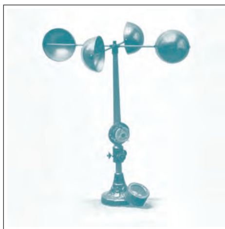
An early anemometer designed by John Thomas Romney Robinson in 1846. (photo by Sean Linehan, NOS, NGS, courtesy NOAA)
