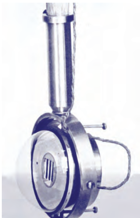
This Angstrom pyranometer from 1930 measured albedo, which is the amount of electromagnetic radiation reflected from the planet's surface. (NOAA)
