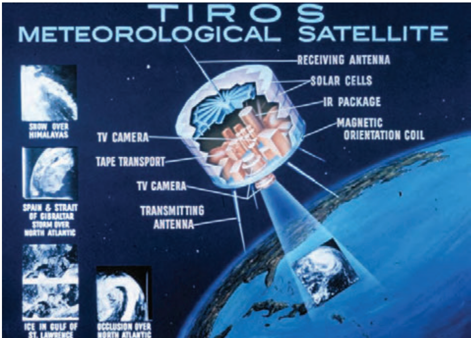
A circa 1961 illustration of TIROS I shows its various components. (NOAA).
