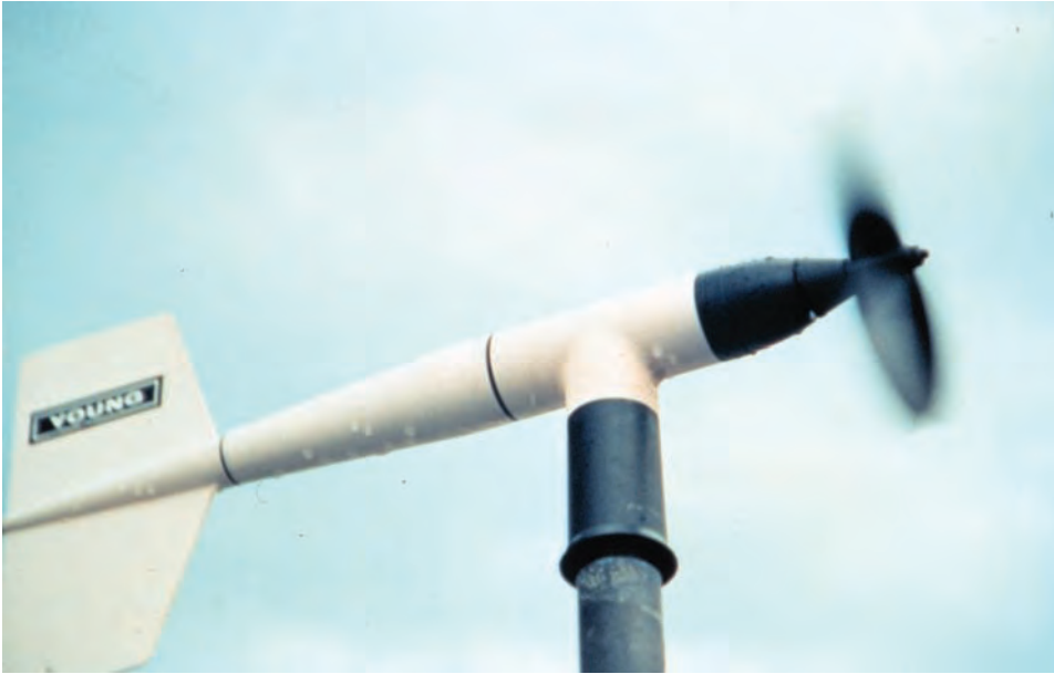
A wind speed instrument mounted on a Project Vortex vehicle monitors conditions in northern Texas in this 1994 photo. (NOAA Photo Library, NOAA Central Library; OAR/ERL/National Severe Storms Laboratory)
