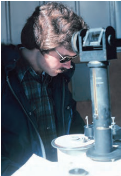
A scientist compares ultraviolet wavelengths at a Mauna Loa, Hawaii, research station using an ozone spectrophotometer. (photo by John Bortniak, NOAA Corps)
