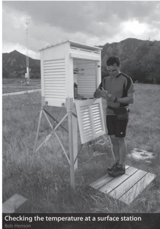
Checking the temperature at a surface station
