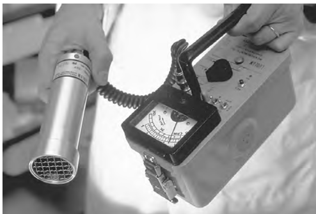
Geiger counters are used to detect subatomic particles emitted by radioactive substances. Hank Morgan. National Audubon Society Collection/Photo Researchers, Inc. Reproduced by permission.
