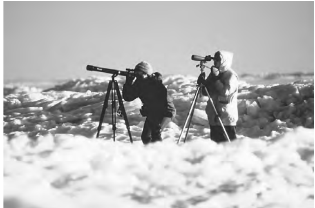
The telescope collects and analyzes the radiation emitted by distant sources. The most common type is the optical telescope, a collection of lenses and/or mirrors that is used to allow the viewer to see distant objects more clearly by magnifying them or to increase the effective brightness of a faint object. Photograph by Robert J. Huffman. Field Mark Publications. Reproduced by permission.
