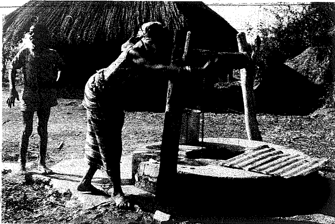
(26) An improved well in Zambia, using a windlass to reduce the effort
