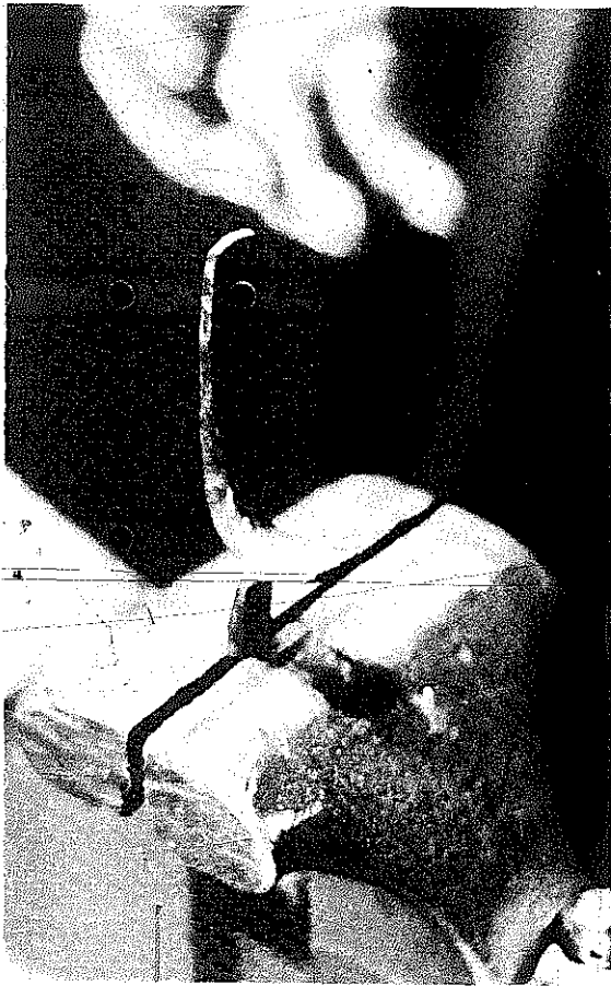
PLATE 281 Hershel has flattened the end of the grip rail and formed a curve for the owner's fingers.
