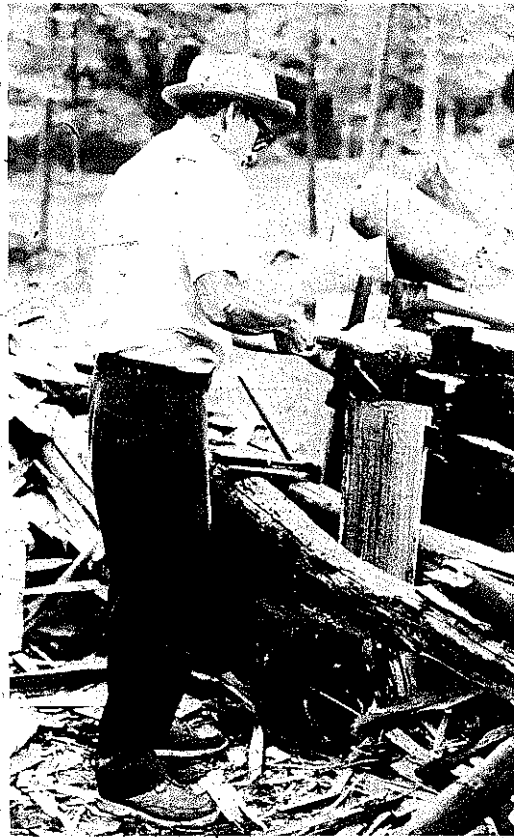
PLATES 111-113 Harley Rogers, demonstrating how to split, or rive, shingles—splitting the "bolt" which will then be split into shingles.
