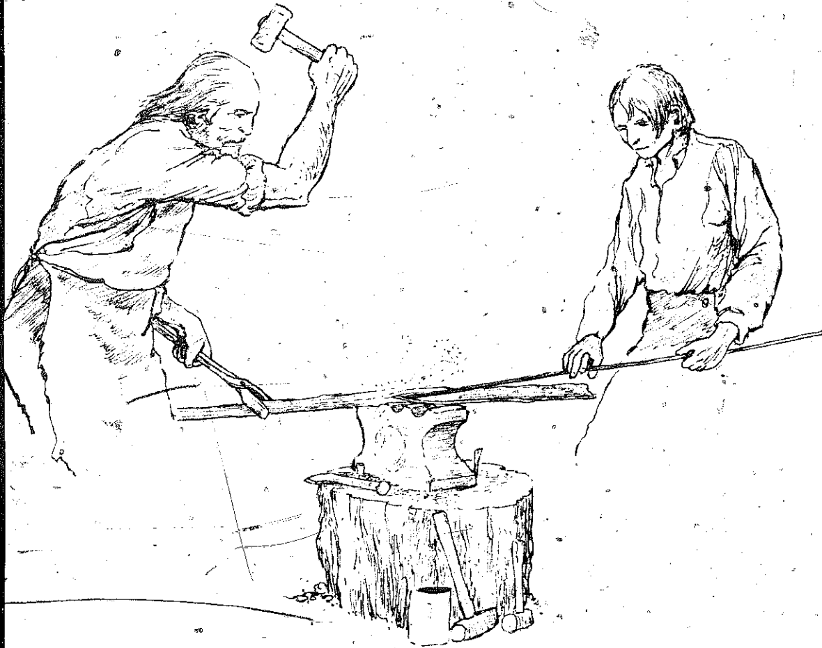
PLATE 174 A gunsmith and his apprentice hand-forging a gun barrel. (Drawing by Hershel House.)
