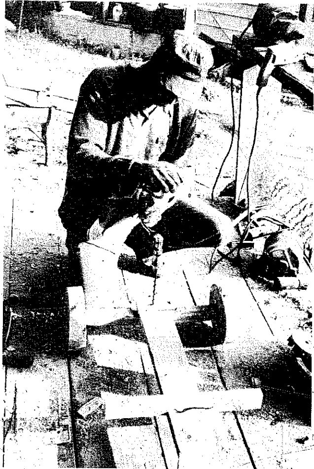
PLATE 280 To complete the front axle assembly, Clyde drills a hole through it for a metal bolt that will hold it together loosely enough so that the front axle will turn with ease.
