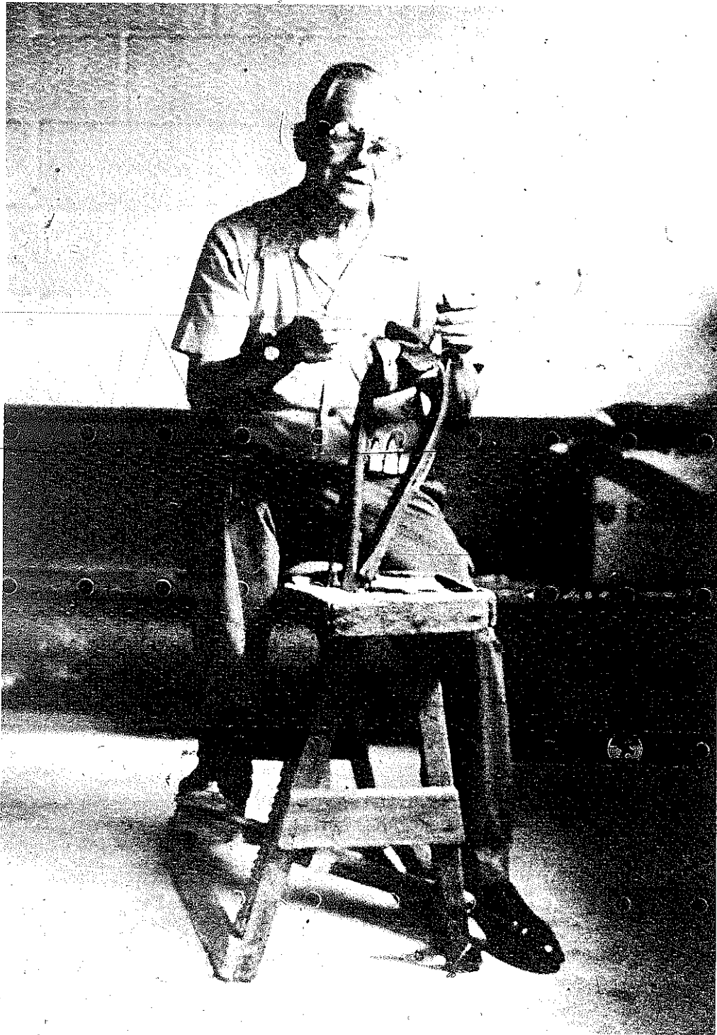
PLATE 120 A stitching horse was usually used to free both hands for stitching and pegging.
