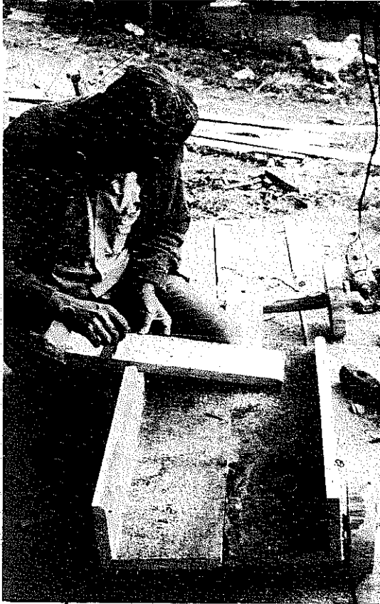
PLATE 282 To complete the bed, Clyde cuts out a back rest and nails it into place at a slight slant behind that portion of the bed that serves as a seat.
