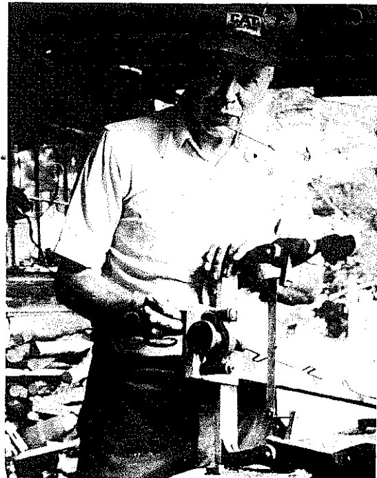
PLATE 321 Clyde readies the end of the shaft with its ball-bearing attachment for the propeller.
