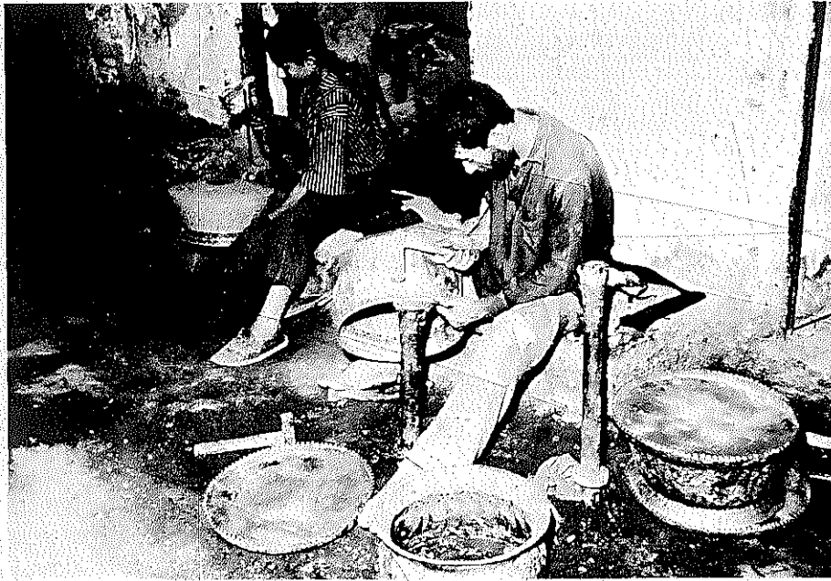
Figure 27 Coppersmiths Planishing (left) and Flanging (right)
