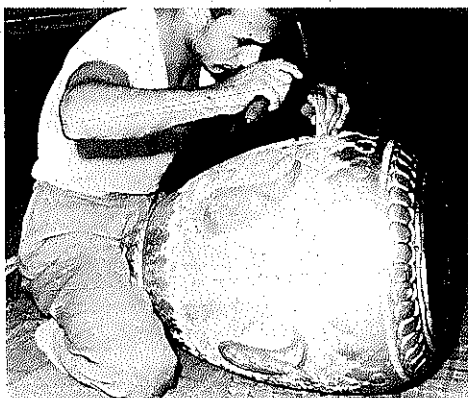
Figure 41. A Metal Embosser Working on a Vessel Filled with Pitch
