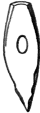
Fig 66—Showing a Faulty Method of Making a Chisel.
