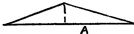
Pointing Cultivator Shovels by the Method of "A. M. B." Fig. 383— Showing the Shape to which the Steel is Drawn.
