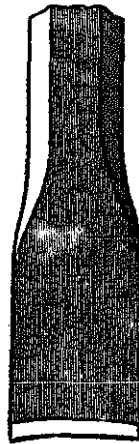
Fig. 48—Improperly Ground Chisel.
