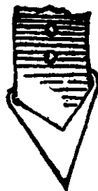
Fig. 389—The Point Adjusted Ready for Welding.
