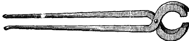
FIG. 101.—TONGS FOR BENDING IRON FLATWISE.
