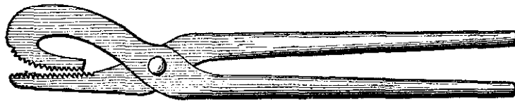
Fig. 182—The Handy Clincher, as made by A. F. Reinbeck.
