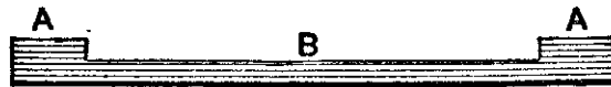
Making a Slot Circle by the Method of "Iron Doctor." Fig. 199—Showing the Shape of the Piece.
