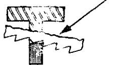
Figure 1-26.—Selecting the proper hacksaw blade.
