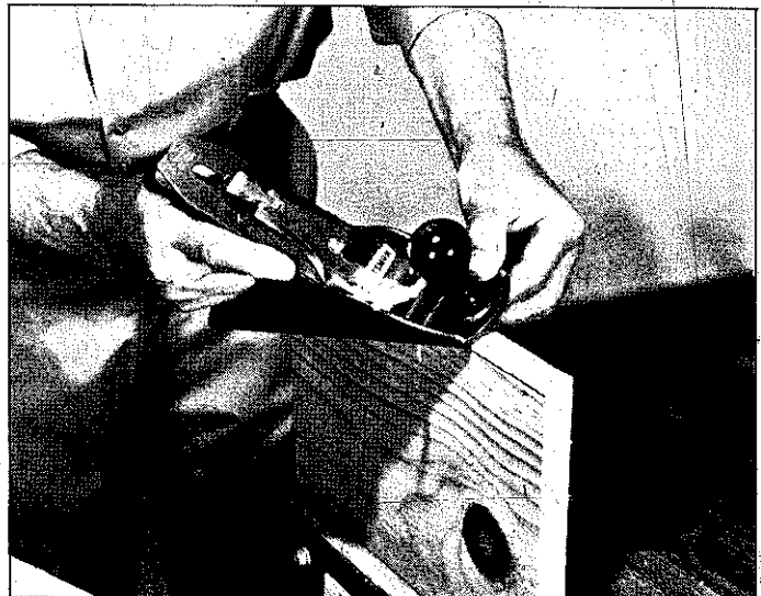
BEVELS or CHAMFERS can be made by holding the plane at the correct angle throughout the pass using your free hand for extra guidance. Carefully mark the edge of the work with a pencil before cutting.
