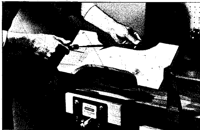
This unusual use of a bar clamp as a vise allows you to change the position of the work easily.
