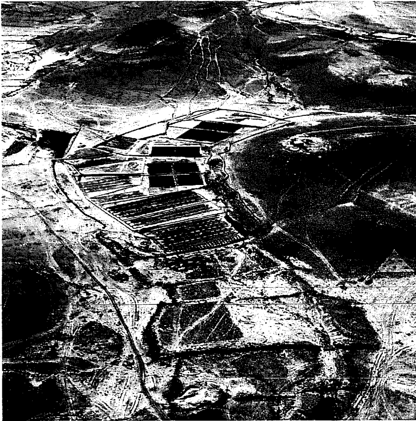
Aerial photograph of the Avdat farm and its watershed. In the foreground: unreconstructed ancient terraces. In the background: on the slopes one can easily identify the channels leading the runoff water to the farm.
