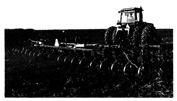
Chisel plowing, a form of conservation tillage, mixes crop stubble into the soil, leaving the ground partially protected from wind and rain. Chisel plowing can reduce erosion by 30
