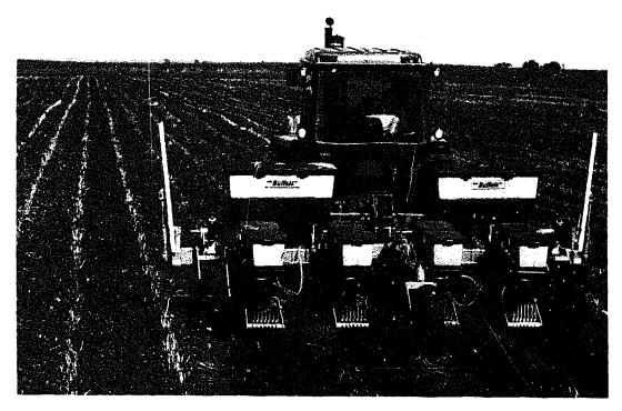
A ridge-tillage planter places seeds in a narrow band of soil scraped off the top of the ridges. This method preserves the residue cover between the rows, reducing soil and water runoff. Planted last fall as a cover crop, hairy vetch helps to meet the nitrogen needs of the corn crop now being planted. *Credit:* Dick Thompson, the Thompson Farm.
