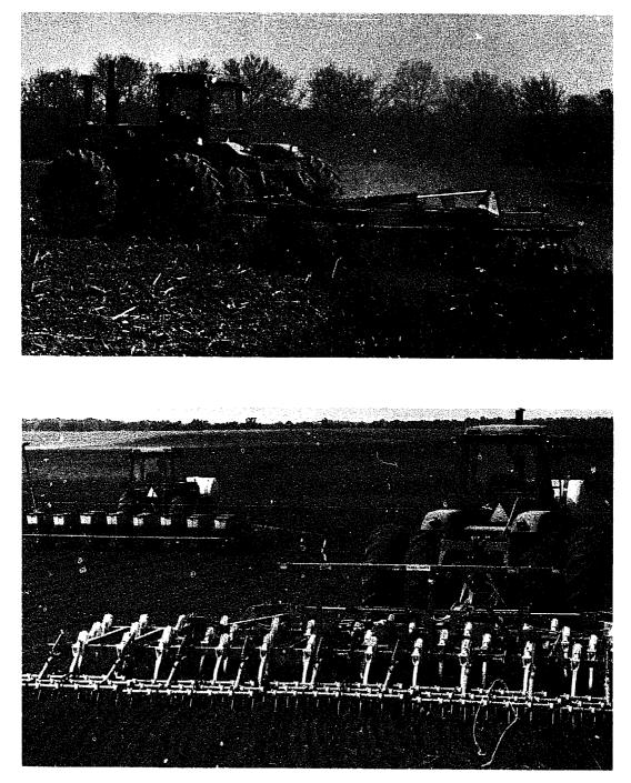
An offset disk is a conventional tillage tool used for further soil preparation (top). Final field preparation is accomplished with a field experience high soil losses if hard spring rains cultivator, which in this case is also incorporating a preplant herbicide into the soil (bottom). At the left, a planter follows. These conventional tillage operations work the soil
