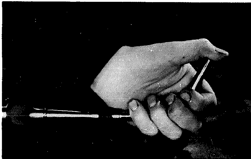
Fig. 14.4. Test the oxygen system for leaks. Top—the eight places numbered should be tested with soapy water while the oxygen system is under pressure. Bottom—open the blowpipe oxygen valve and hold the thumb over the end of the tip to put the oxygen passages under pressure.
