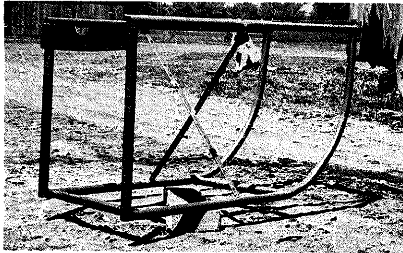
Fig. 13.31. A barrel stand, which makes the tilting of a barrel easy. (Constructed by Joe Rosenstiel, Illinois.)
