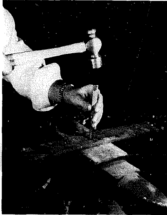
Fig. 4.75. The location of a hole to be drilled should be marked with a center punch.
