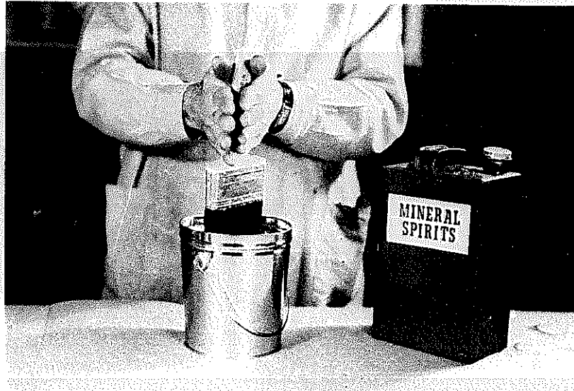
Fig. 11.3. After cleaning a paint brush, remove the liquid in the brush by twirling the handle between your hands.
