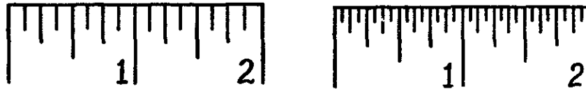
Fig. 4.14 Examples of two graduations frequently found on rules such as the foot ruler, yardstick, zigzag rule, folding rule, pull-push rule, and tapes. The graduations on the rule to the left are eighth-inch, and the graduations on the rule to the right are sixteenth-inch.
