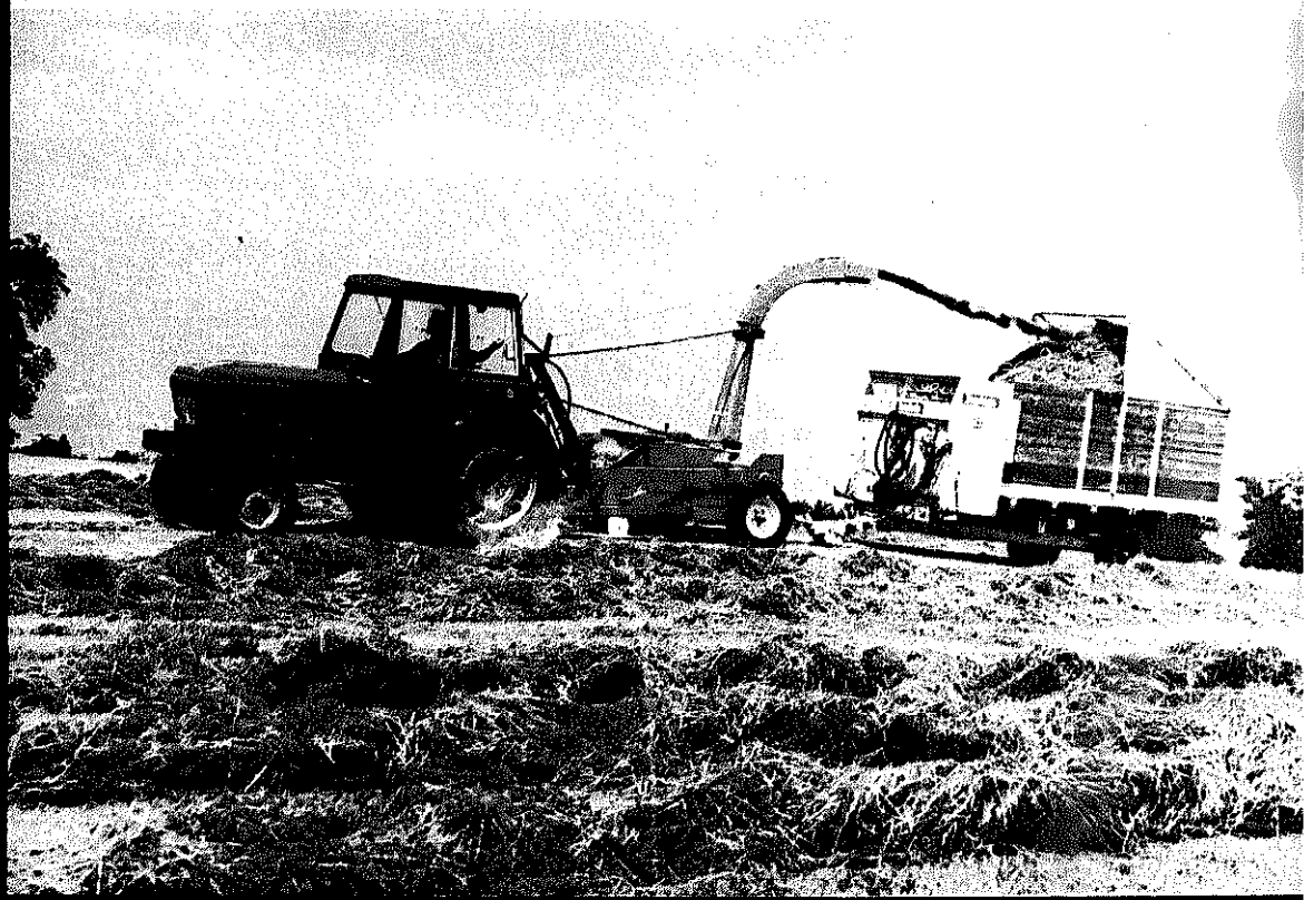
Plate 28 A Bamford forage harvester cuts, pulverizes and blows the grass into a trailer
