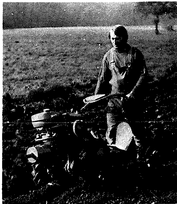
Agria 6000 with weighted wheels for extra traction to pull a reversible moldboard plow. Agria-Werke
