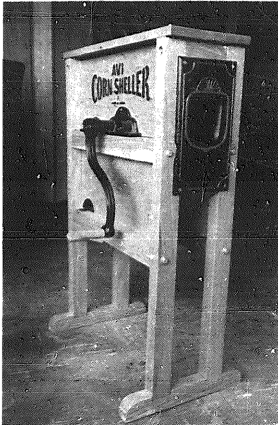
The AVI Cornsheller, showing the hand crank and corn exit. On the other side of the sheller, a large flywheel gives each stroke momentum.
