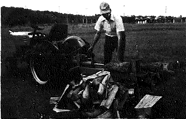
Mounted on a three-point hitch, this hydraulic attachment for the Power King Tractor splits logs up to 26 inches in a 15-second cycle. Engineering Products Co.
