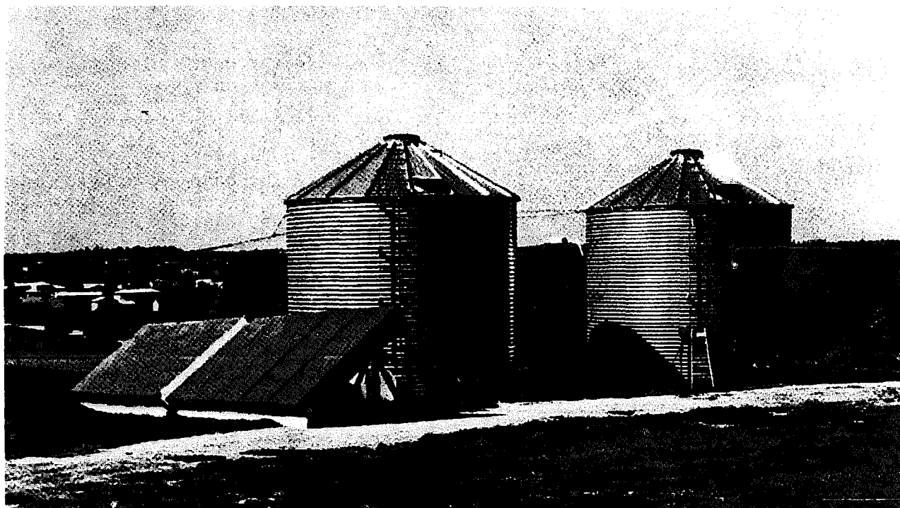
Figure 3 Portable Flat-Plate Solar System used in corn drying experiment, located at U.S. Grain Marketing Research Center, Manhattan, Kansas
