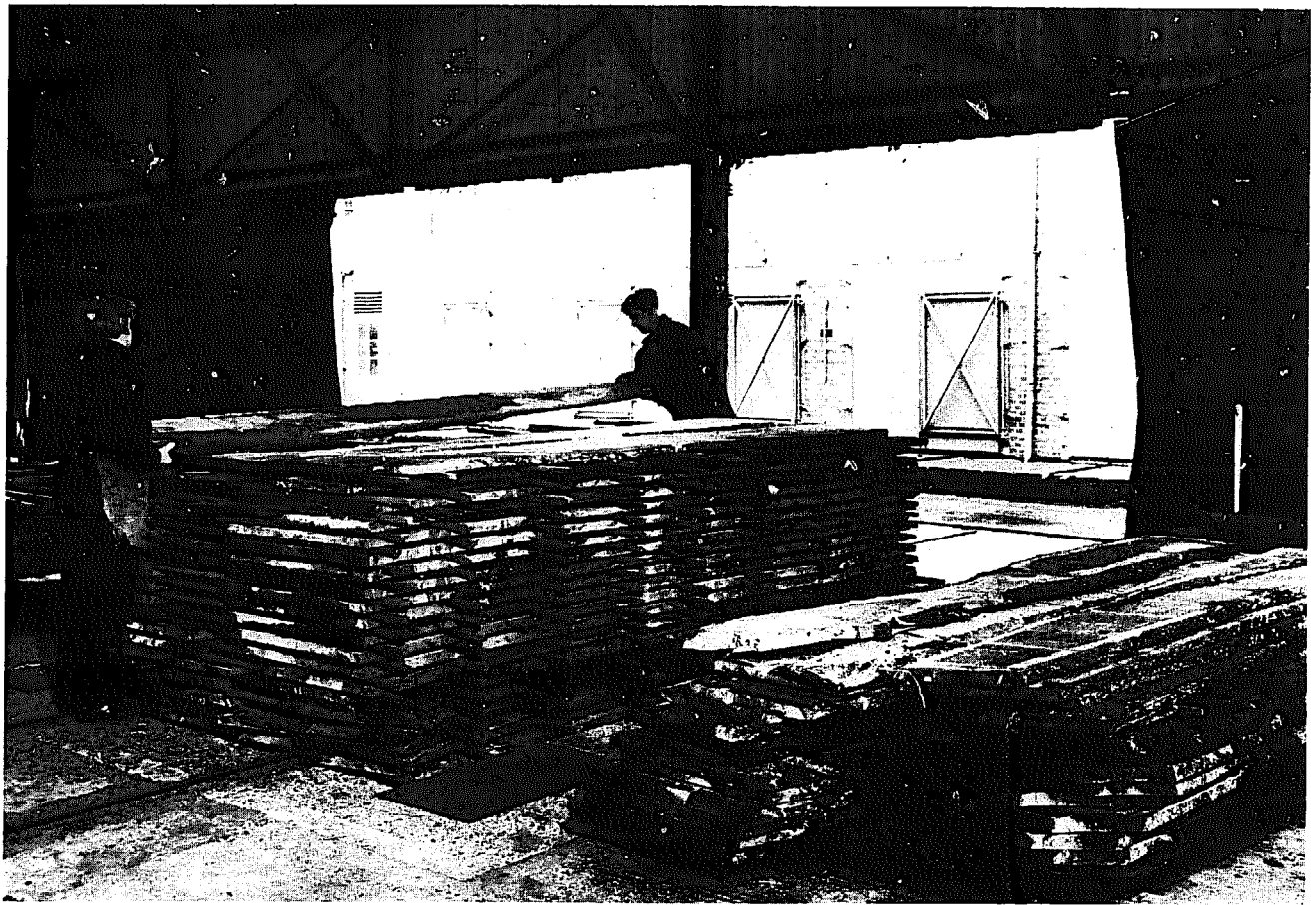
Plate 30 Piling stack on a lumber lift
