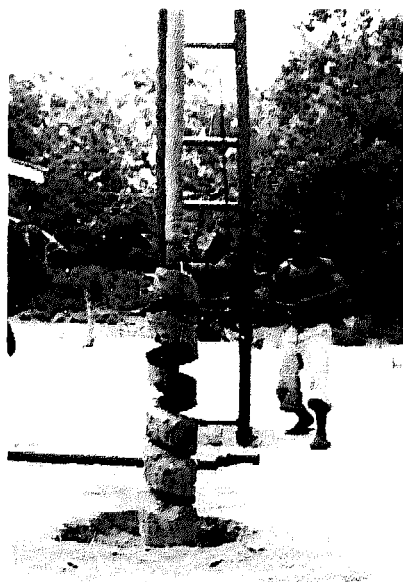
Fig. 68. The equipment will not be overloaded if the flight auger is not filled over more than 0.5 m.
