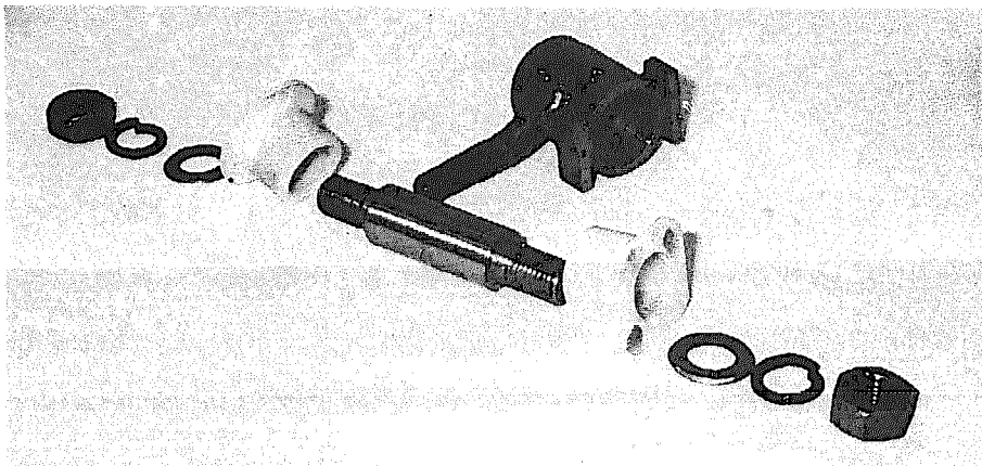
FIGURE 3 FULCRUM AND HANGER ASSEMBLIES FOR ACETAL BEARINGS
