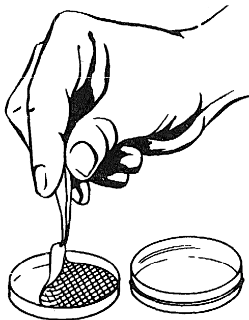
Fig. 13. Placement of Membrane on Pad Soaked With Culture Medium
