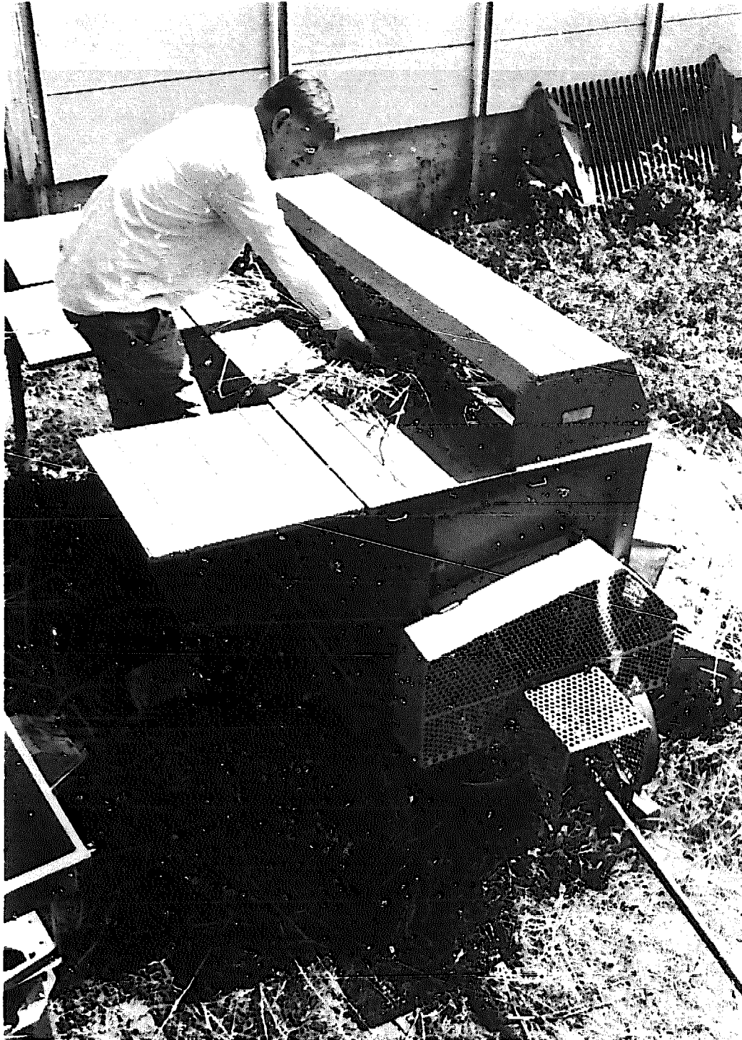
Fig. 5 - Thresher in use with work-table in position.
