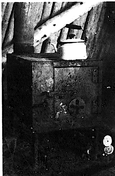
Figure 17.3 (left) —Sheet-steel stove with cast-iron stove top and feeder door. Collection of Pete MacManus.
