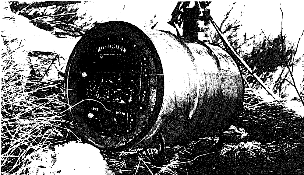
Figure 16.2—Horizontal whole-barrel stove made with a barrel-stove kit from Fatsco. Note how a No. 10 can fits perfectly over the stovepipe collar at the rear. Made by Howard Kantner.
