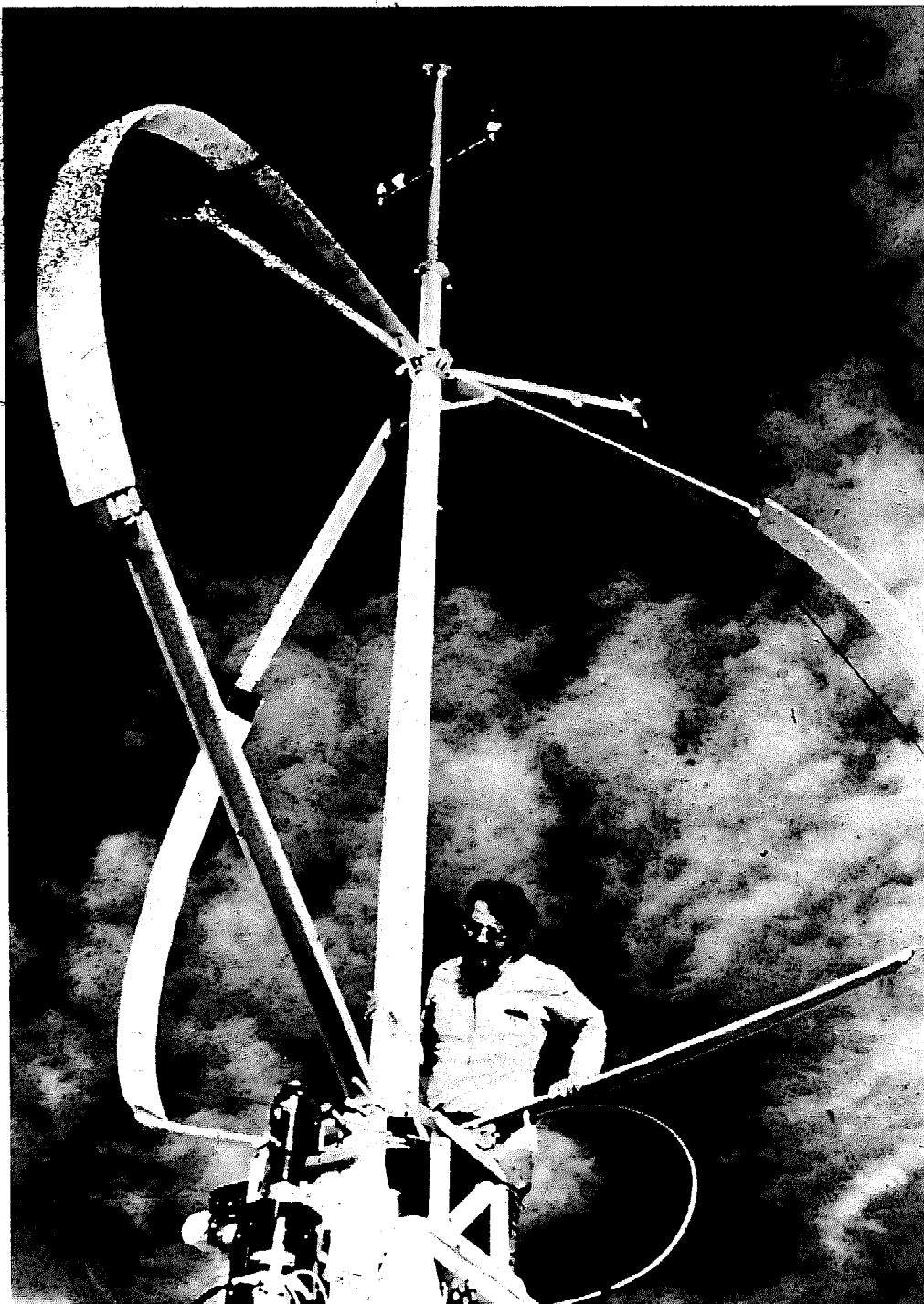
Eggbeater-style Darrieus rotor being tested at Sandia Laboratories in Albuquerque, New Mexico. This high-performance machine uses extruded aluminum blades.
