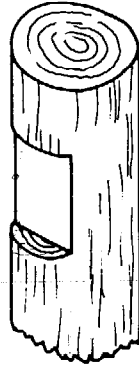
FIGURE 53 ROUND POLE NOTCHED FOR SAWN FRAMING MEMBER.
