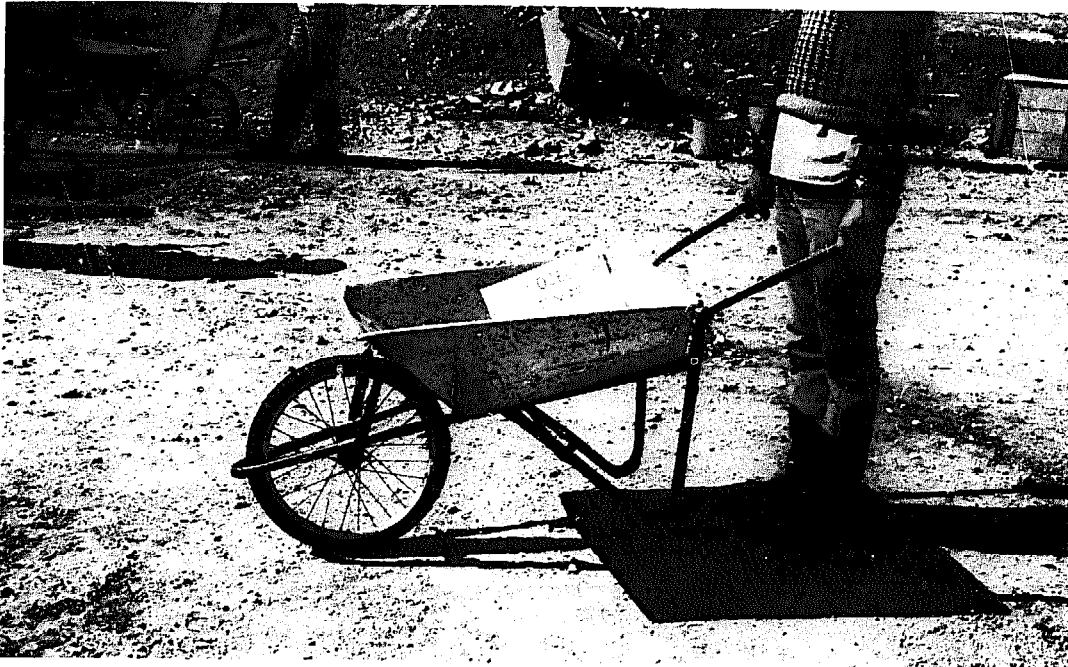
a) One-Wheel Barrow with Light Wrought Iron Tube Frame and a Pneumatic Tired Cycle Wheel (Type E)
