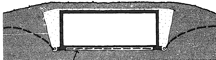
GRAVEL BACKFILL GIVES LOW RISE TO WATER TABLE AND STOPS CAPILLARY DRAW
