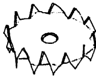
Figure 4.10 Double sided Toothed Plate connector.
