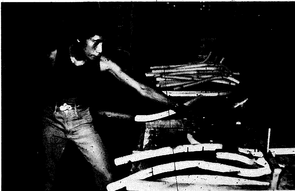
Figure 38. Adjusting shaped components with the aid of a kerosene fired blow torch
