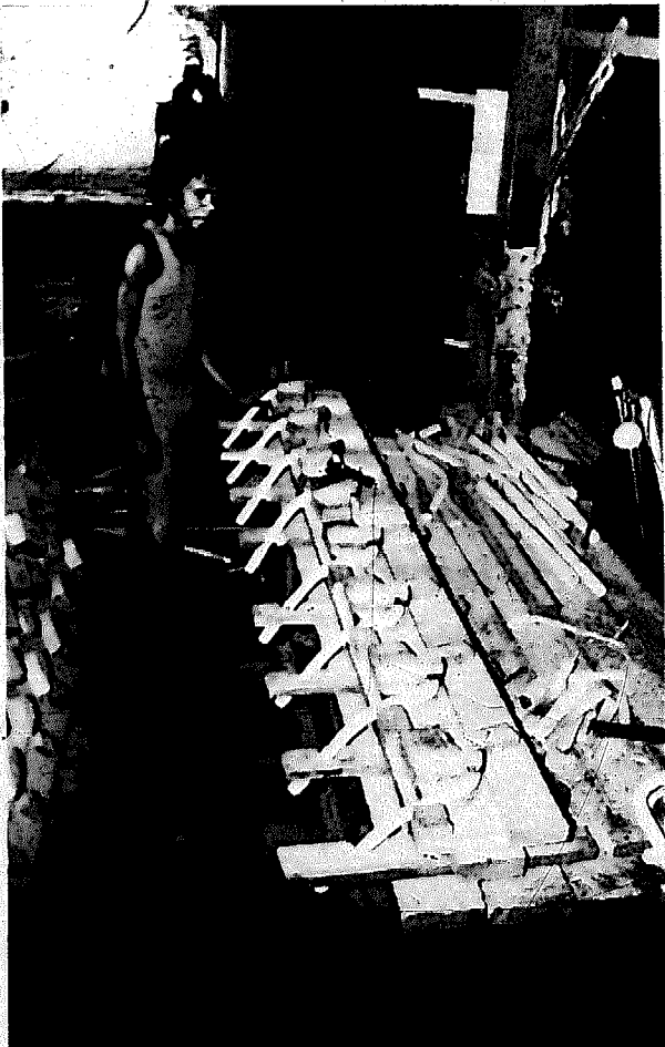
Figure 28. Loaded moulding jig for compound moulds
