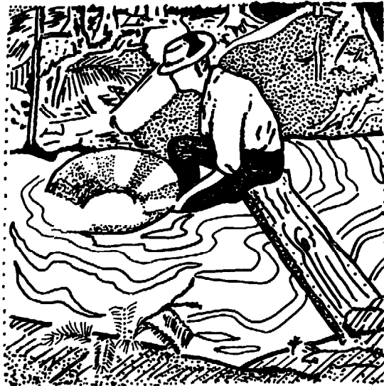
Fig. 8 Concentration of material with a batea
