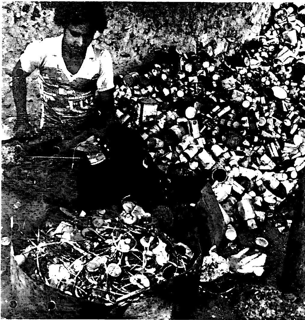
Fig. 34 Shearing open used cans. The thin strip contains solder. If the material were sent for detinning, this would be removed. Egypt.
