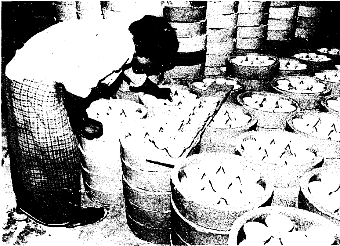
Fig. 2-125: Cups are set in saggars outside the kiln.
