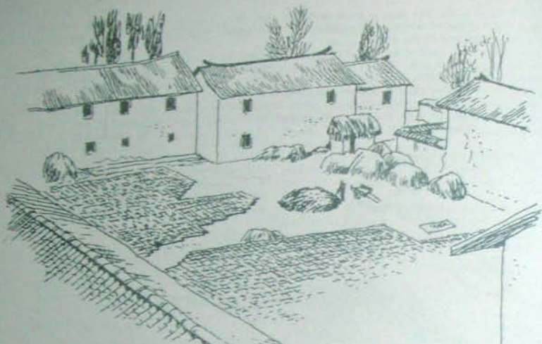
Looking down onto the farm with the bricks laid out to dry. The heap of mud is in the centre and the handcart used to move it. To the right is the mat on which the mud is placed.
