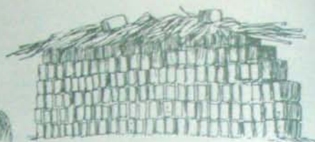
Stack is running protected with maize stalks.
