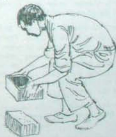
The mould was lifted to reveal the newly made brick.
