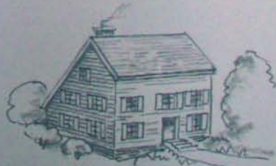
New England Saltboxes open to the sunny south with a high front wall while minimizing exposure to cold north winds. (Cold Humid climate)
