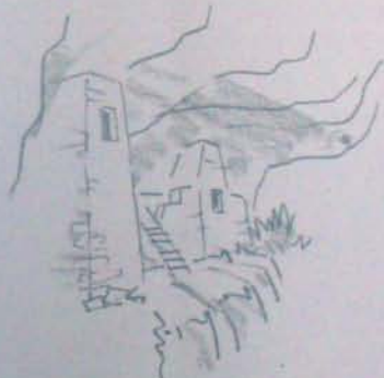
Mesa Verde Cliff Dwellings, carved into the side of a canyon, are warmed by the sun. The south-facing cliff blocks cold winter winds, and the rock walls and floors store the sun's heat for cool evenings. (Hot Dry climate)
