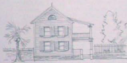
Charleston Two-Story, Side Porch Houses are one room wide to catch cooling sea breezes. The two-story porch creates shade and extends the living space into the gardens. (Hot Humid climate)
