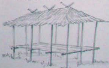
Elevated Pole Houses in the tropics stand above the damp ground and allow cooling breezes to circulate freely. A thick roof provides shade and insulation from the solar heat. (Hot Humid climate)
