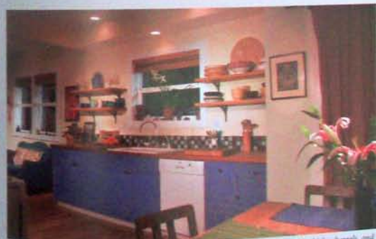
Colorful wheatboard cabinets, salvaged oak flooring, a countertop made from old whiskey barrels, and shelves that were once bleacher seats combine to make a lively, functional kitchen between the living and dining areas.
