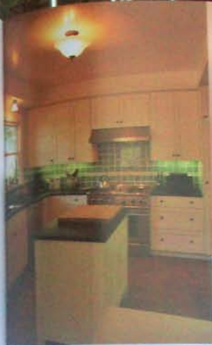
Fluorescent task lighting directly on the work surface helps improve a kitchen's energy efficiency.
